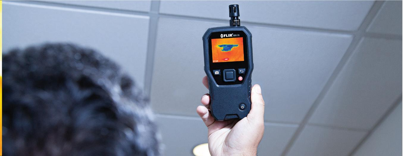
Featuring IGM technology powered by a built-in thermal imaging sensor, the MR176 and MR160 can visually guide you to the precise spot that moisture may be hiding.
