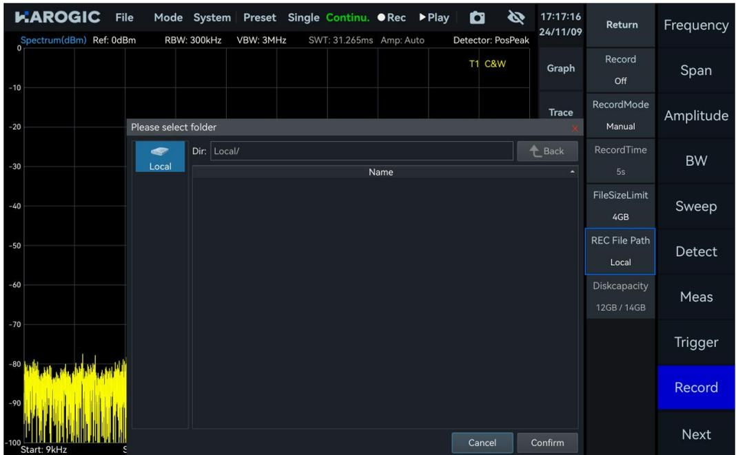
In Fixed Duration Mode, click "Record on" to automatically record the preset amount of data. In Manual Mode, click "Record on" and "Record off" to manually control the recording duration. The recording will automatically stop when the file size exceeds the available disk capacity.
