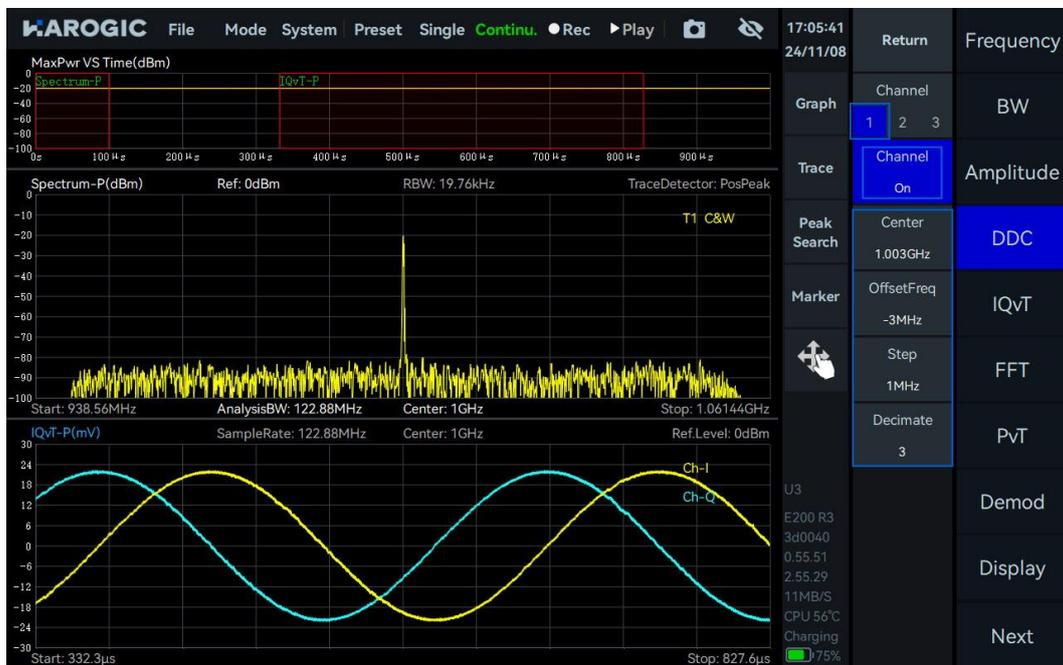
3. Click "FFT" in the main settings area, select "DDC1 Channel" from the dropdown menu, enable "Analyze", drag the red selection box "Spectrum-D1" in the maximum power time thumbnail, or adjust the "TimeStart" and "TimeLength" values to perform spectrum analysis on the sub-IQ streams generated by the DDC at different time intervals.
