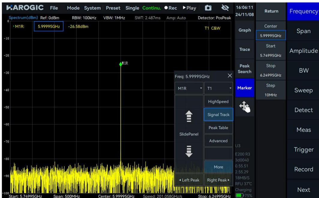
Note: Generally, this function only moves the frequency position and does not change the span. However, for signals with a particularly large drift that exceed the current span, tracking becomes difficult. For signals at the edge of the instrument's sweep range, the span will be further reduced due to frequency limitations.
