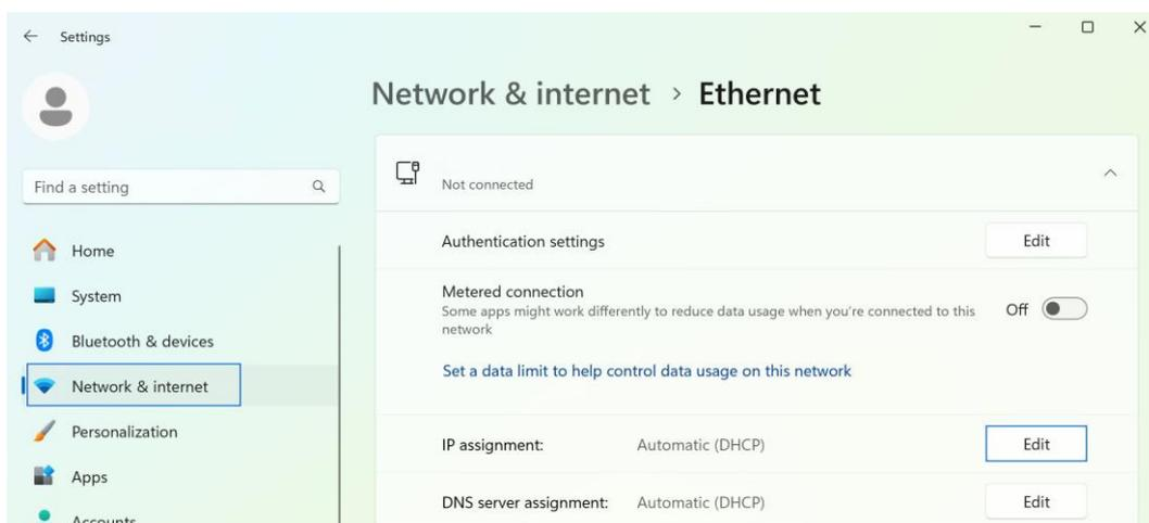
6. Select "Manual" to set IP, turn on the IPv4 option, and set the IP address and subnet mask (the computer IP and the instrument IP must be in the same network segment). For example, set the computer IP address to 192.168.1.2 and the subnet mask to 255.255.255.0;
