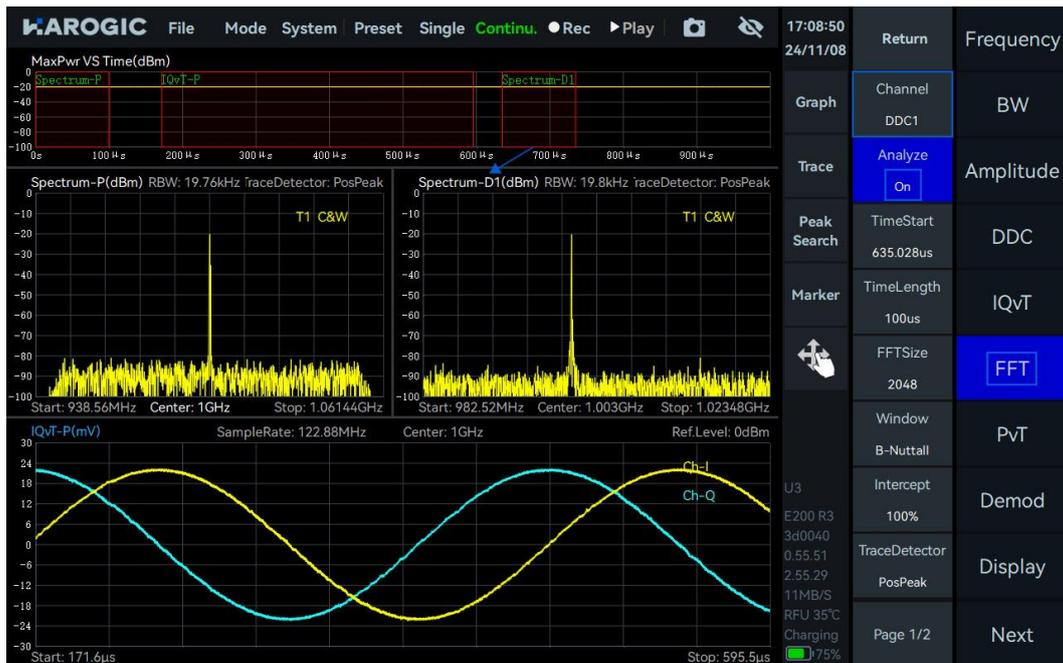
4. Click "IQVT" in the main settings area, select "DDC1 Channel" from the dropdown menu, enable "Analyze", drag the red selection box "IQVT-D1" in the maximum power time thumbnail, or adjust the "TimeStart" and "TimeLength" values to perform time-domain analysis on the sub-IQ streams generated by the DDC at different time intervals.
