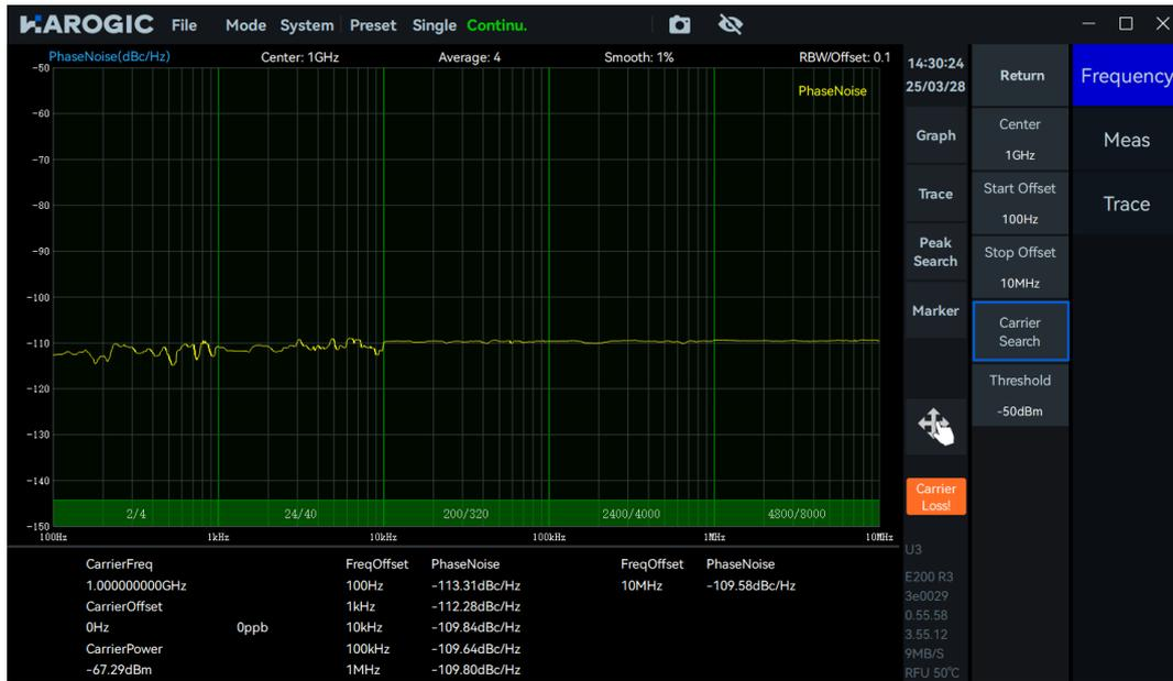
2. After locating the carrier signal, refer to the [Phase Noise Measurement of Known Carrier Information](#) section to set the start frequency offset and end frequency offset for phase noise measurement.
