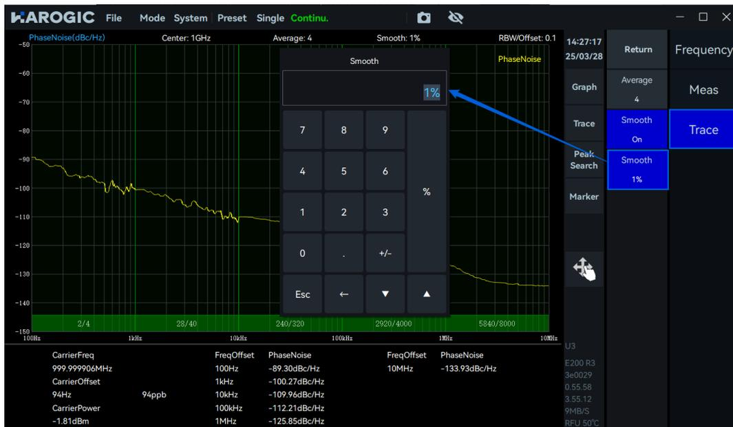
4. The instrument will automatically complete the phase noise measurement within the set frequency offset range, and the measurement results are shown below. In the phase noise measurement table at the bottom of the interface, you can obtain the carrier information and the phase noise values of each characteristic frequency offset point (unit: dBc/Hz).
