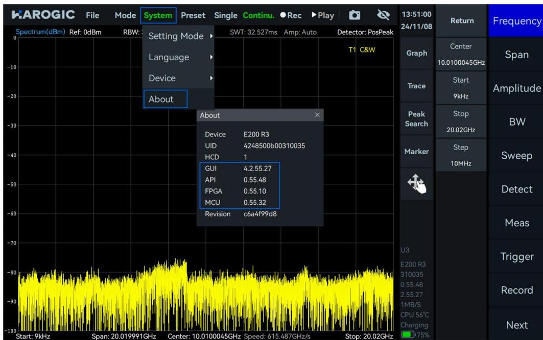
After firmware updates, you need to ensure that the instrument's MCU firmware, FPGA firmware, and SASStudio4 software (API) are in the same major version. Different major versions are incompatible with each other. For example, they must be 0.55.x to work properly.
