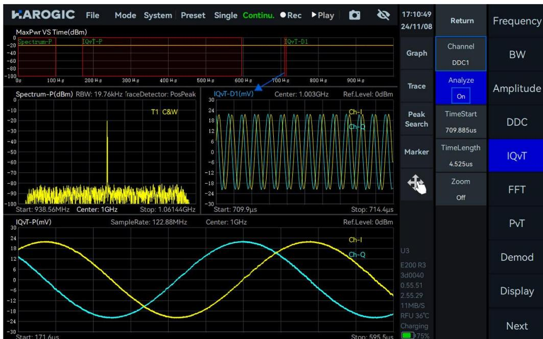
5. Click "PvT" in the main settings area, select "DDC1 Channel" from the dropdown menu, enable "Analyze", drag the red selection box "PvT-D1" in the maximum power time thumbnail, or adjust the "TimeStart" and "TimeLength" values to perform power vs. time analysis on the sub-IQ streams generated by the DDC at different time intervals.
