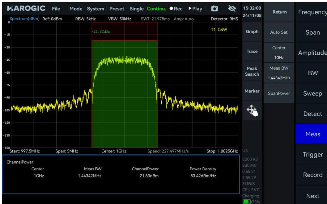
3. You can also manually adjust the channel center frequency (drag to select the measurement area) and the measurement bandwidth (drag the measurement border left or right or adjust the Meas BW settings).
