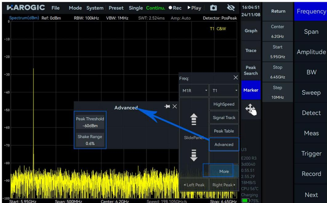
2. Click "Signal Track". The reference marker will search for peaks within the current sweep span and align the peak signal to the center frequency position. When the target signal frequency drifts, the spectrum analyzer will automatically adjust its center frequency so that the signal always remains in the center of the display area, facilitating user observation and analysis.
