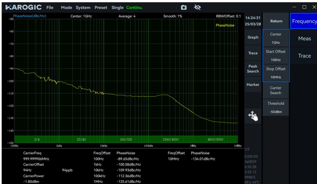
2. If there is strong jitter at the near end of the signal under test, click "Meas" in the main settings area, then select "Detection Settings" in the additional menu. In the pop-up window, appropriately increase the frame detection rate of the corresponding frequency band to obtain more convergent measurement results;
