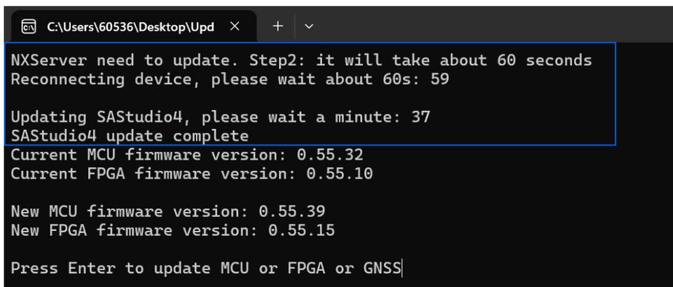
4. After the SASstudio4 software is updated, the program will display the current instrument firmware version and the new firmware version in the update program. After confirming that they are correct, press Enter to start the update. (In the following, Updater 0.55 M39F15 is used as an example. M39 is MCU 0.55.39, and F15 is FPGA 0.55.15).
