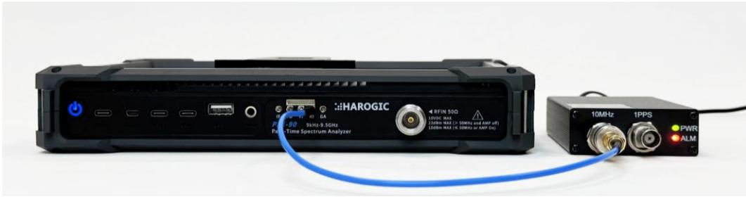
2. Click "Next"->"System" in the main setting area, set the reference clock frequency "RefCLKFreq" to 10 MHz, and select "External" for the reference clock source "RefCLKSource". If the reference clock source displays "External", it means the switch is successful. If the reference clock source rebounds to "Internal" and an error pop-up window appears, it means the switch failed. At this time, you can click "Preset" to switch back to the internal clock.
