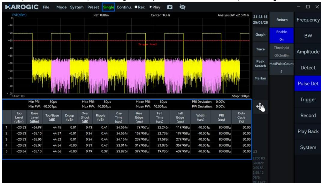
6. If the user encounters a measurement freeze/stop state during pulse detection, this can be avoided by reducing the analysis bandwidth or increasing the pulse period.
