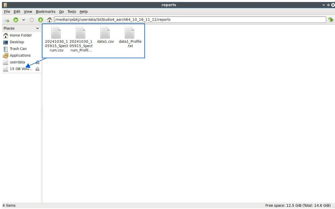
8. Copy the instrument calibration to "..\SASStudio4\bin\CalFile" on the PC, double-click "SASStudio4.exe" under "SASStudio4\bin" on the PC to open the SASStudio4 UI to achieve remote control of the PX series instruments.
