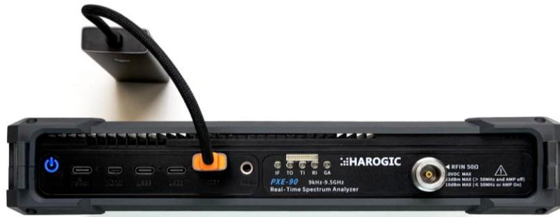
2. Connect the expansion dock to the network port of the computer or embedded instrument via a network cable;
