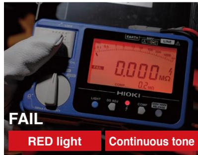
Compare measured values to pre-set reference values to generate a pass or fail decision with the Comparator function.
