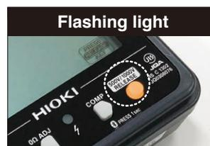
Under [500V], [1000V], or [PVΩ] settings, the RELEASE button will blink. Press to unlock the release of high voltages as an extra safety measure.
