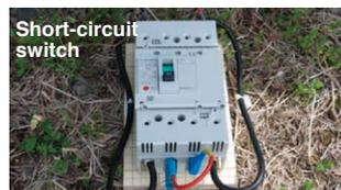
Normally, to accurately measure the insulation resistance of a generating PV, one needs to short the measured circuit. That's not necessary with the IR4053.
