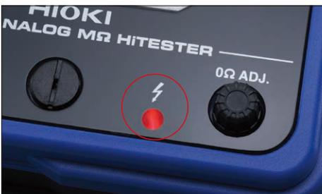
The LIVE CIRCUIT LED will light up in red whenever the voltage exceeds 20 V AC between the LINE and EARTH terminals, and when at least 20 V DC is still remaining during the auto discharge.
