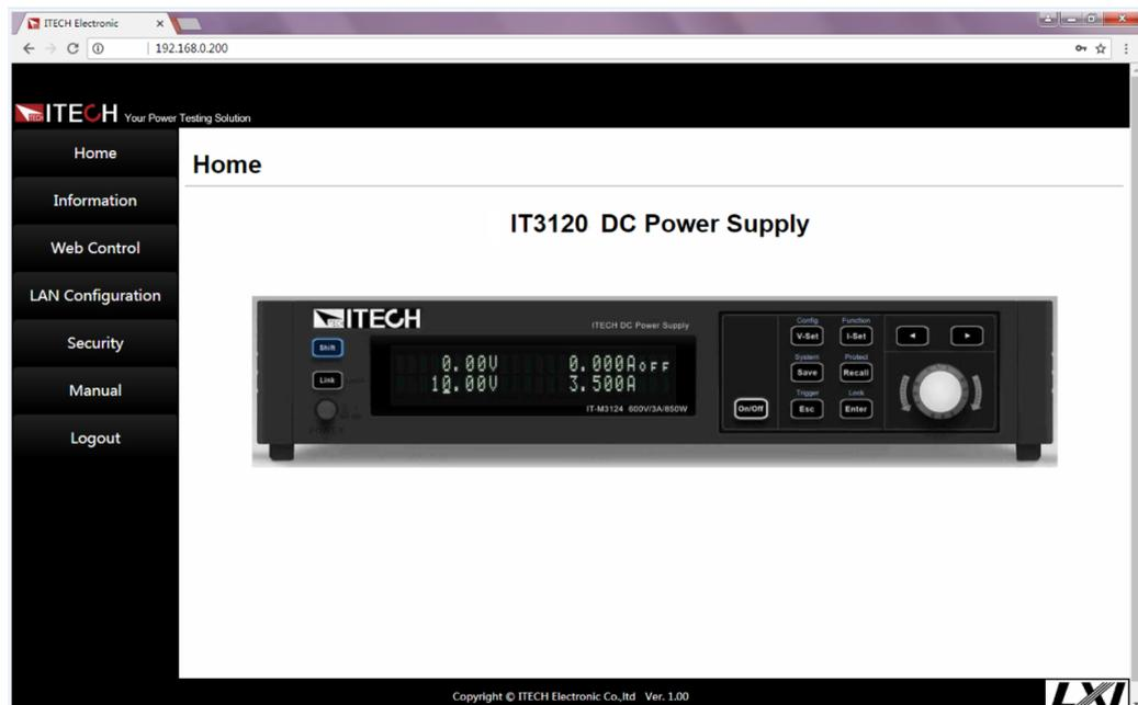
You can select different interfaces by clicking the seven buttons shown in the navigation bar on the left side of the window. The detailed descriptions are as follows.
