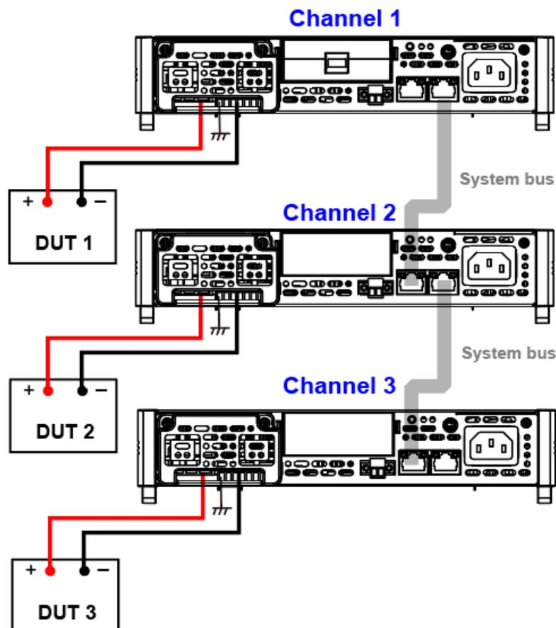
1. Configure the channel number of each instrument. Please refer to [8.1 Multi-Channel Function](#) for detailed introduction.
