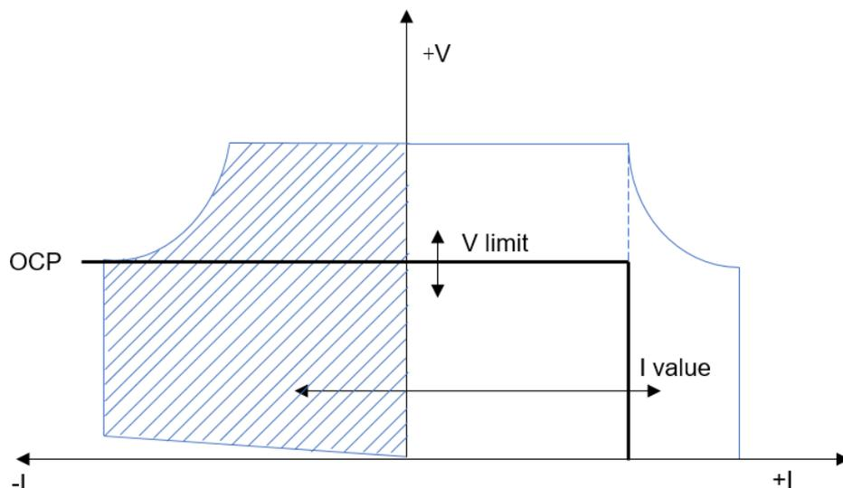
The heavy solid line illustrates the locus of possible operating points as a function of output. As shown by the vertical portion of the line, the output current remains regulated at its programmed setting as long as the output voltage remains within its limit setting. A CC (constant current) status flag indicates that the output current is being regulated and the output voltage is within its limit settings.
