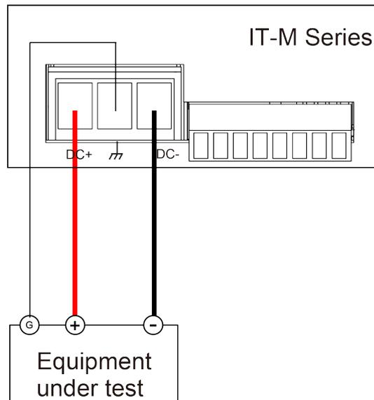
1. Confirm that the power switch is in the OFF position and verify that there is no dangerous voltage on the connection terminals.
