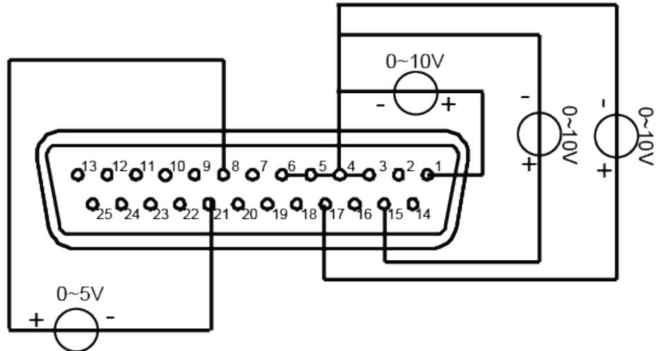
When 0V is input, the instrument's On/Off state is switched to Off state.
