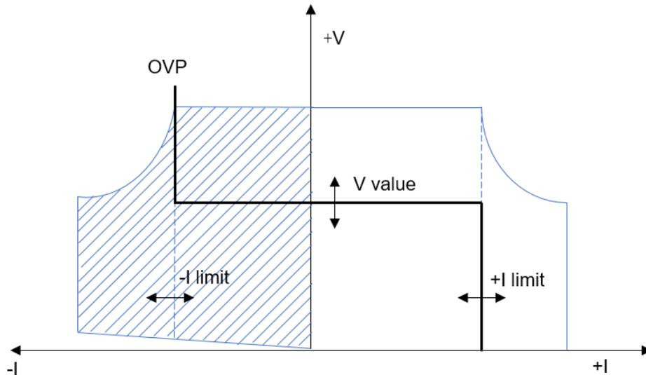
The heavy solid line illustrates the locus of possible operating points as a function of output. As shown by the horizontal portion of the line, the output voltage remains regulated at its programmed setting as long as the load current remains within the positive or negative current limit setting. A CV status flag indicates that the output voltage is being regulated and the output current is within its limit settings.
