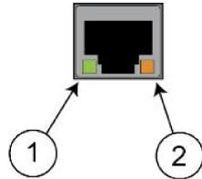
If neither of the LEDs is lit, the network is not connected.
