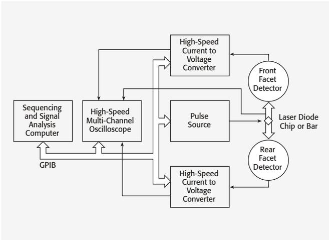
**FIGURE 1.** This schematic reflects the current testing practices of major laser diode manufacturers. Note that the use of discrete test components increases the integration and programming effort, while severely limiting the flexibility of the test system.
