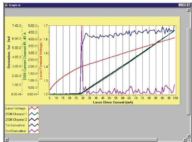
**FIGURE 3.** This plot illustrates the Model 2520’s pulsed LIV sweep capability. The sweep was programmed from 0 to 100mA in 1mA steps. Pulse width was programmed at 1µs at 1% duty cycle, providing for a complete sweep in just 10ms (excluding data transfer time).
