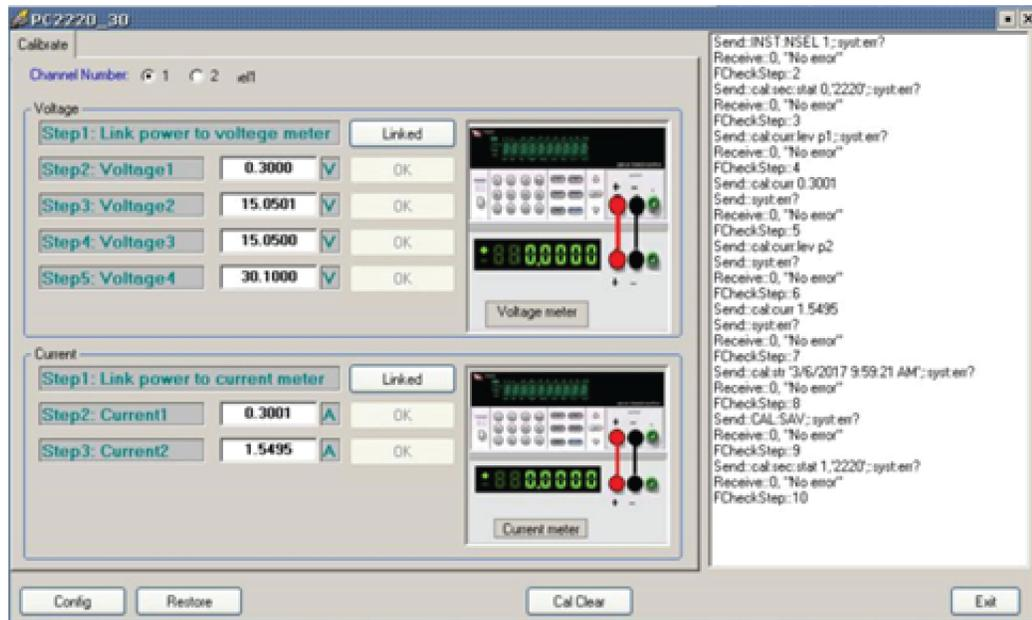
4. Click the **Linked** button in the software. **Step 2** is selected (the software sets up the instrument to a voltage depending on the DUT).
