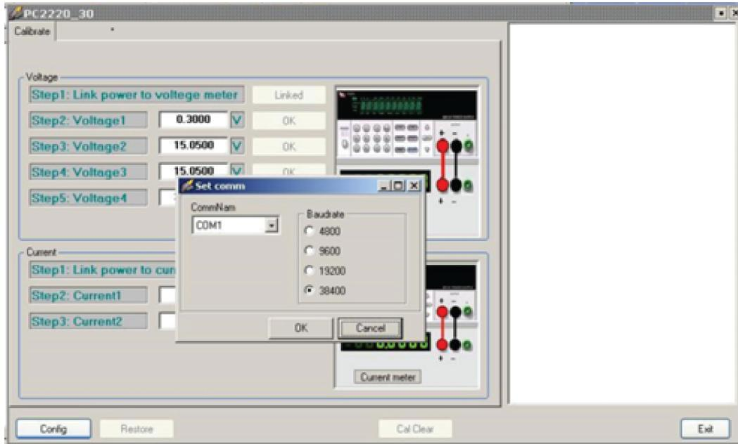
3. Click the **Linked** button in the software. The right pane of window should indicate INST:NSEL 1:system? and the response "No error".
