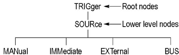
You can create commands and queries from these subsystem hierarchy trees. Commands specify actions for the instrument to perform. Queries return measurement data and information about parameter settings.
