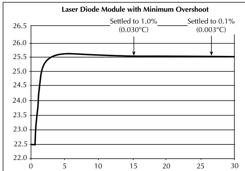
B. For a 3°C step: Settled to  $\pm 1.0\%$  ( $\pm 0.030^\circ\text{C}$ ) in 15.32 seconds
