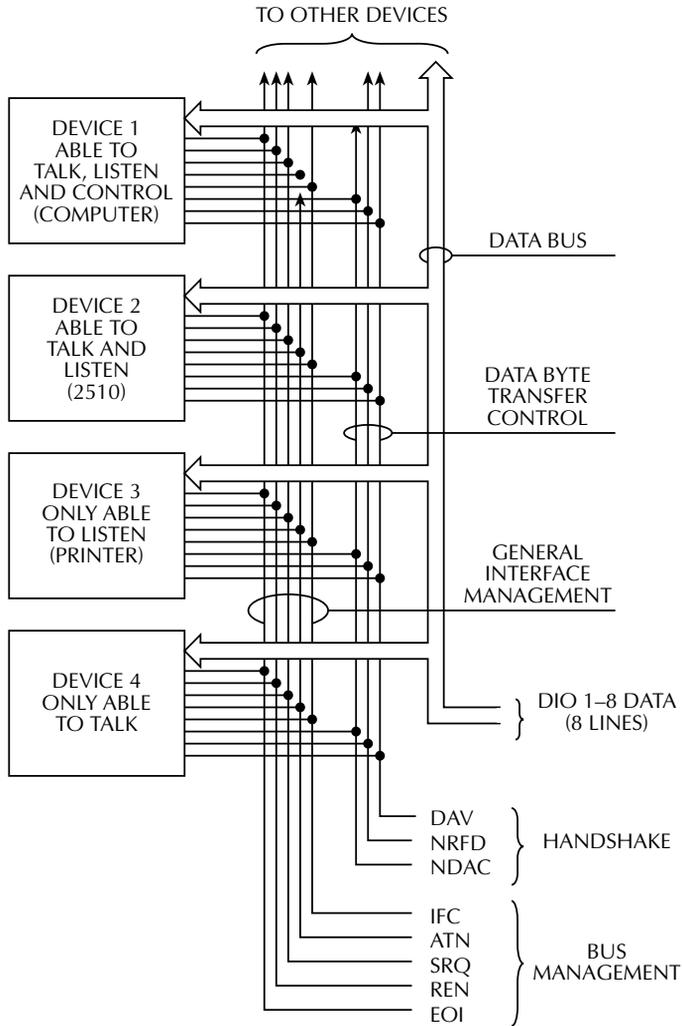
There are two categories of controllers: system controller and basic controller. Both are able to control other instruments, but only the system controller has the absolute authority in the system. In a system with more than one controller, only one controller may be active at any given time. Certain protocol is used to pass control from one controller to another.
