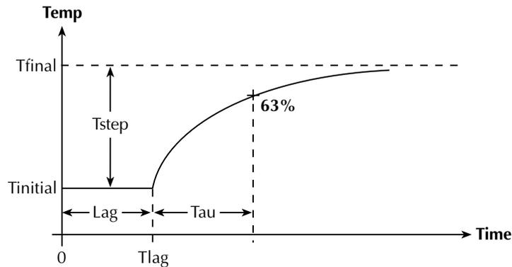
In this case  $T_{\text{step}}$  is positive, but it could also be negative. Temperature responses of a different mathematical model will cause the autotune function to fail (or give unpredictable results). Once the Lag and Tau times are extracted from the sampled data taken from the voltage step response, the tuning constants can be calculated. Inherent limitations that will cause the tuning function to fail include:
