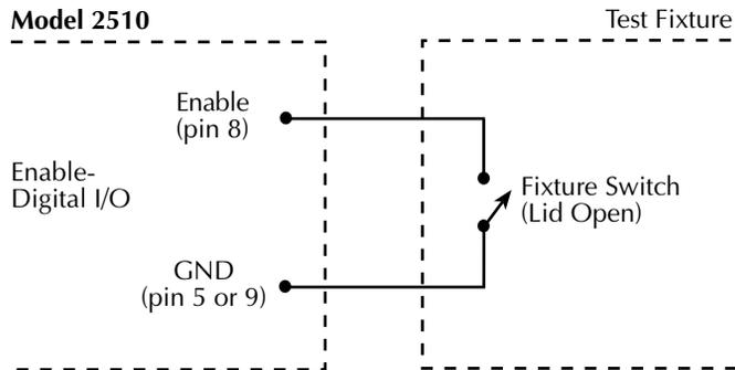
**B. 2510 OUTPUT turns off and cannot be re-enabled until closed again.**
