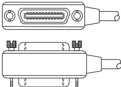
To allow many parallel connections to one instrument, stack the connectors. Two screws are located on each connector to ensure that connections remain secure. [Figure 6-2](#) shows a typical connecting scheme for a multi-unit test system.
