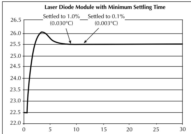
A. For 3°C step: Settled to  $\pm 1.0\%$  ( $\pm 0.030^\circ\text{C}$ ) in 8.54 seconds
