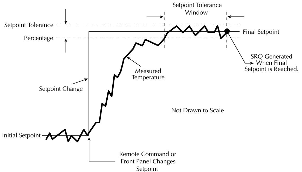
**NOTE** Setpoint tolerance SRQs can be used to generate a temperature sweep. See [Appendix E](#) for details and an example program.
