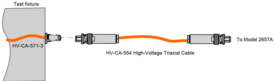
The HV-CA-571-3 is supplied with one unterminated end. It is intended to be used in a safe enclosure.
