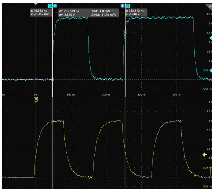
3. Use Multipurpose Knobs **A** and **B** to move the cursors, or touch and drag a cursor. Cursors show readouts that show position and difference measurements between the cursors.
