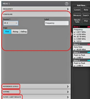
4. Use the available fields to refine the measurement conditions. Displayed fields depend on the measurement. Selection changes take effect immediately. Selection changes can also change fields in other panels.
