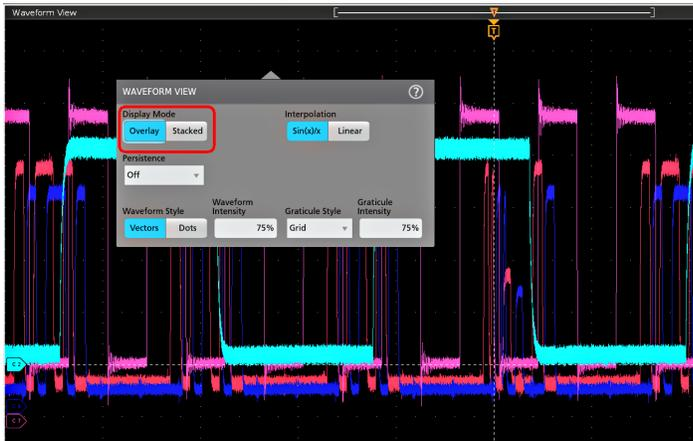
3. Use the other controls to set the waveform interpolation algorithm, waveform point persistence, style, and intensity, and graticule style and intensity.
