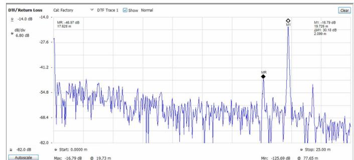
Return loss vs distance for a cable with an inserted barrel and an extension cable. The point at M2 (17.638 m, MR) is the barrel connector and the point marked by M1 at 19.725 m is the end of the cable.
