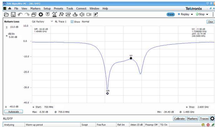
Return loss of a bandpass filter measured from 700 MHz to 2.6 GHz. Markers have been placed a 1.48 GHz (-34.4 dB return loss) and at 1.73 GHz (-11.68 dB return loss), indicating the best and worse match in the passband of the filter.
