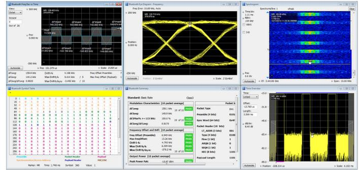
Pass/Fail results are provided with customizable limits. Measurement below shows deviation vs. time, frequency offset and drift and a measurement summary with Pass/Fail results.
