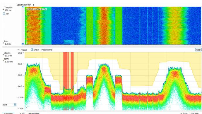
Direction finding and signal strength measurements are quick and easy with the standard SignalVu-PC software. In the illustration below, using the recommended 3rd party Alaris smart antenna, a compass continuously monitors antenna direction while the signal strength monitor performs measurements and provide audio indication of signal strength. When combined with the MAP option for SignalVu-PC, signal strength and azimuth are automatically placed on the map of your choice.
