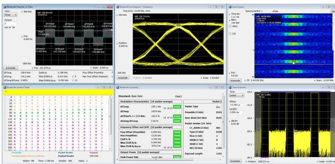
Pass/Fail results are provided with customizable limits. Measurement below shows deviation vs. time, frequency offset and drift and a measurement summary with Pass/Fail results.
