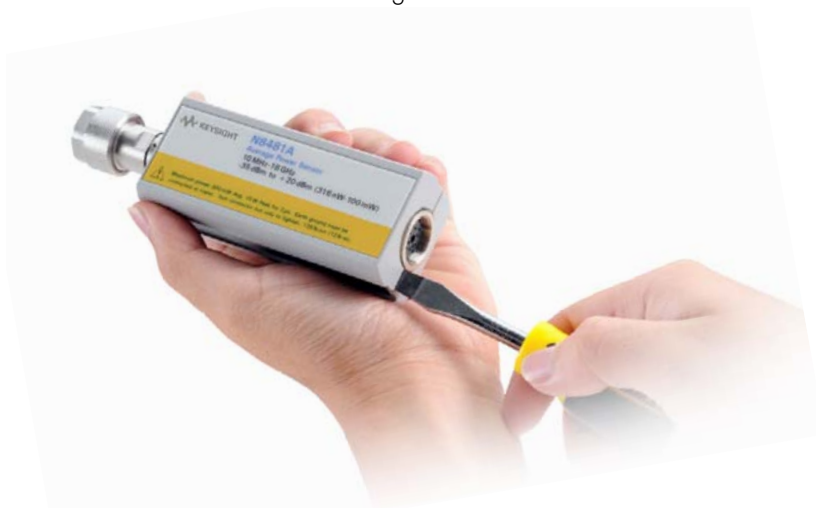
Figure 3-2 Removing the power sensor shell
