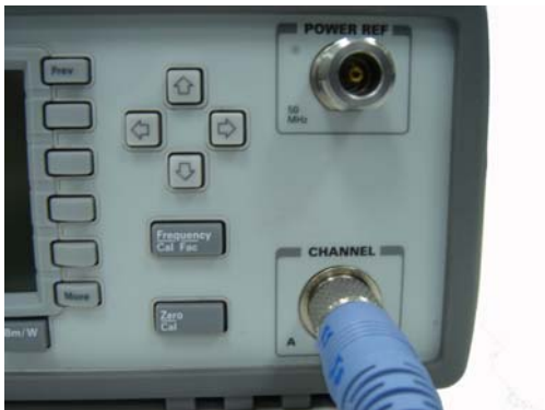
Figure 1-1 Connecting a sensor cable to power meter
