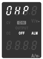
Fig.2-8 ALARM indication example (OHP)
