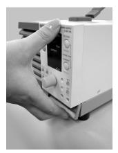
Fig.7-5 Removing the louver
