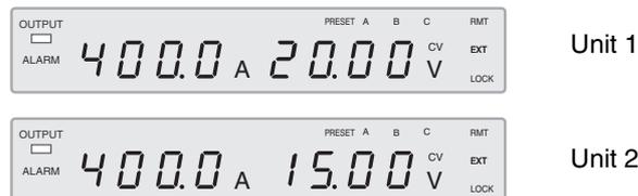
Fig.4-7 Panel display example during series operation
