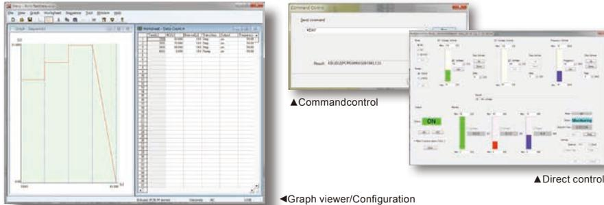
Wavy is an application software that supports sequence creation and the operation for Kikusui power supplies and electronic loads.
