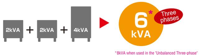
\*8kVA when used in the "Unbalanced Three-phase"
