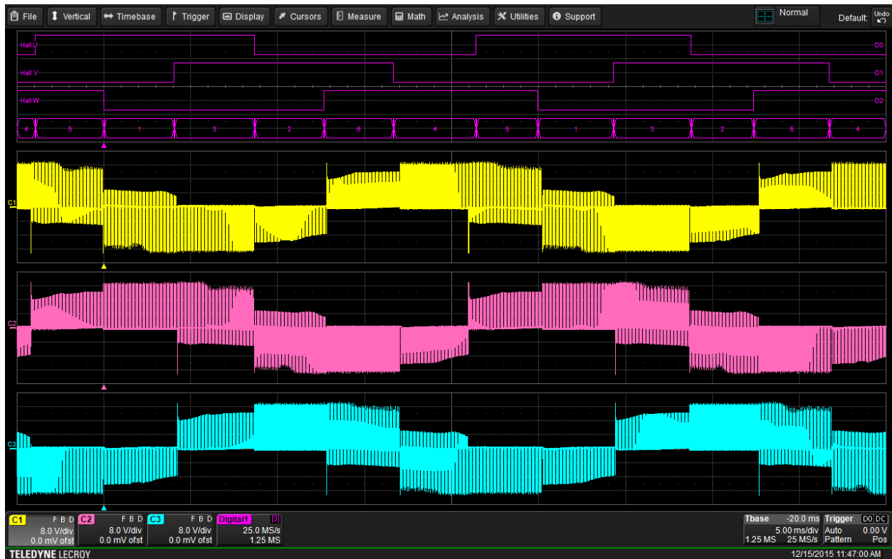
Figure 188: Hall-effect sensor signals and voltage output envelopes are measured again, but with the voltage probed line-to-line.
