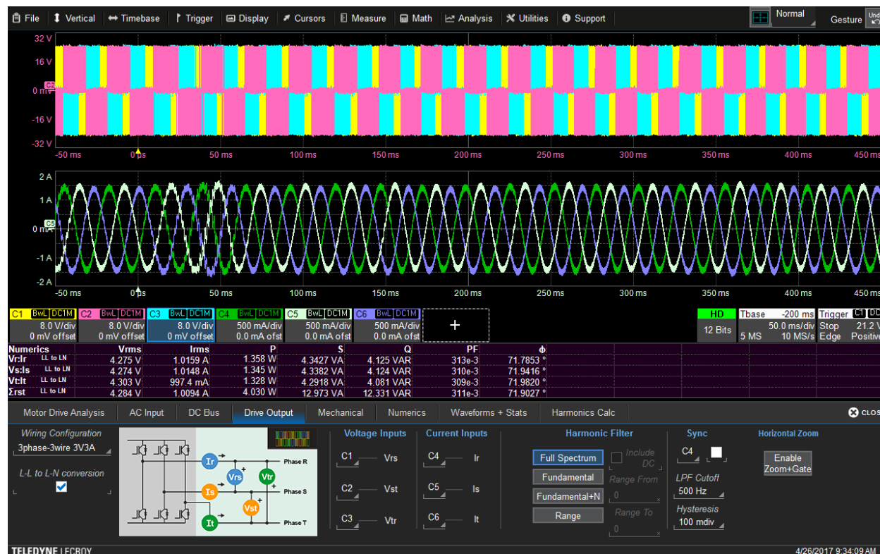
Figure 168: Numerics data calculated for the Full Spectrum of the captured waveform.
