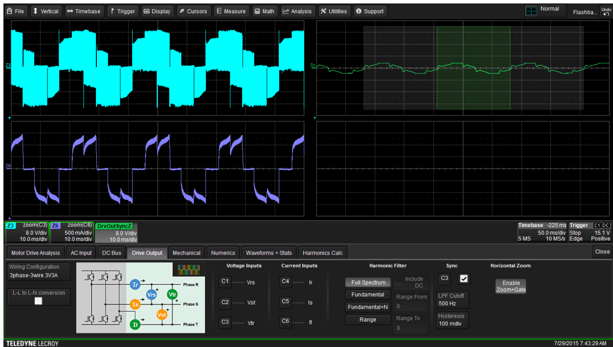
Figure 154: Even with the low-voltage BLDC six-step commutated drive output line-to-line voltage measured here, we can still obtain an accurate Sync signal from this line-to-line voltage signal using the default settings for the low-pass filter and hysteresis.
