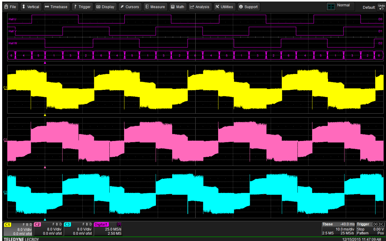
Figure 138: Line-to-line six-step commutated voltages signals together with their three Hall sensor signals.
