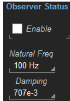
Figure 199: Configuring the MDA for use of the Angle Tracking Observer algorithm.
