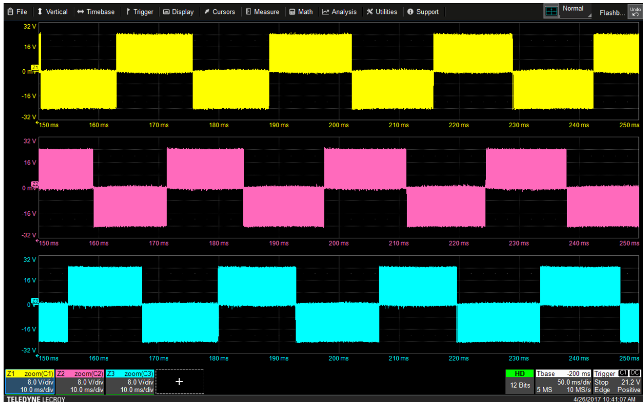
Figure 102: With the load connected as shown in the previous figure, the cascaded H-bridge produces three line-to-line outputs.
