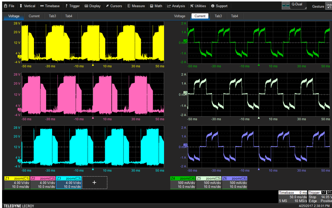
Figure 135: Six-step commutation control produces the motor drive line-to-reference output voltages (waveforms on left) and currents (waveforms on right) shown here. The back-EMF influence from a nearby (energized) phase on the adjacent (non-energized) phase results in the “ramp up” or “ramp down” of the peak voltage, and thus the trapezoidal shape.
