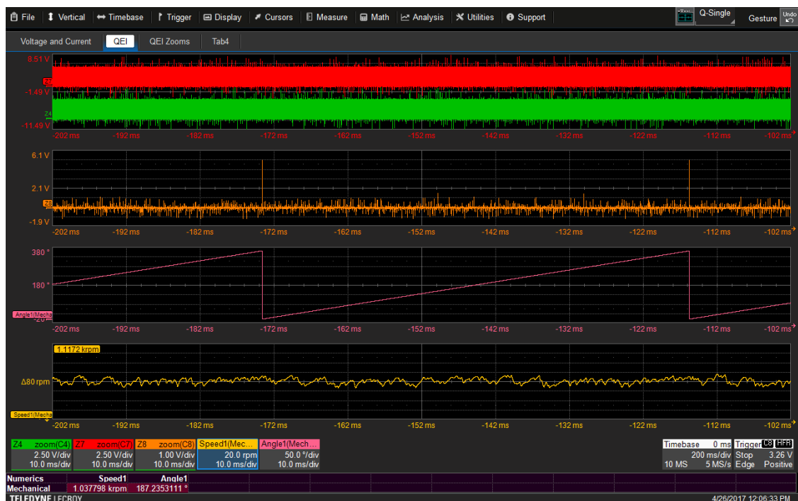
Figure 195: The MDA calculates speed and angle values from QEI signals, displaying the results as waveforms and as well values in the Numerics table.
