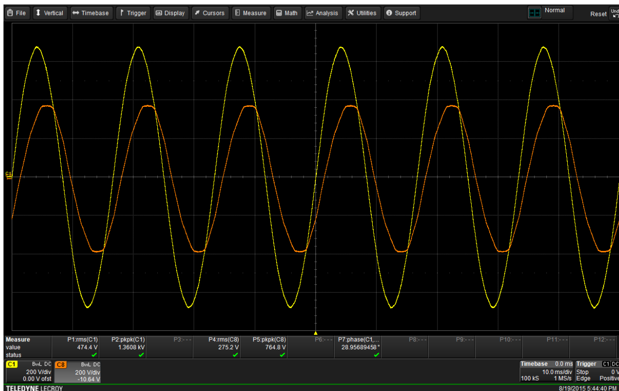
Figure 33: Comparing the magnitude of a line-to-line voltage ( V_{A-B} on ch 1) in a 480-V three-phase system with a line-to-neutral voltage ( V_{A-N} on ch 8).
