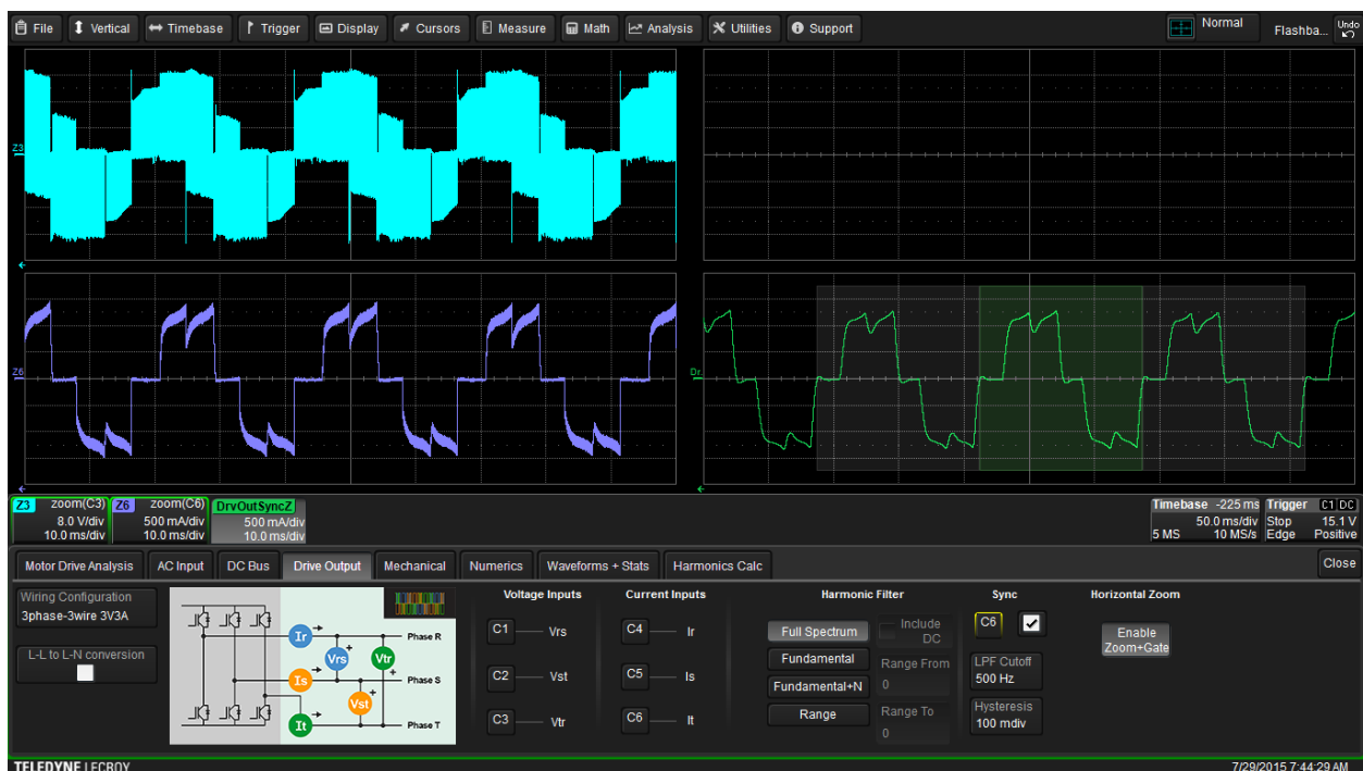
Figure 155: Choosing the line-current signals as the Sync signal for the low-voltage BLDC six-step commutated drive output produces similar results to those obtained in Fig 8.
