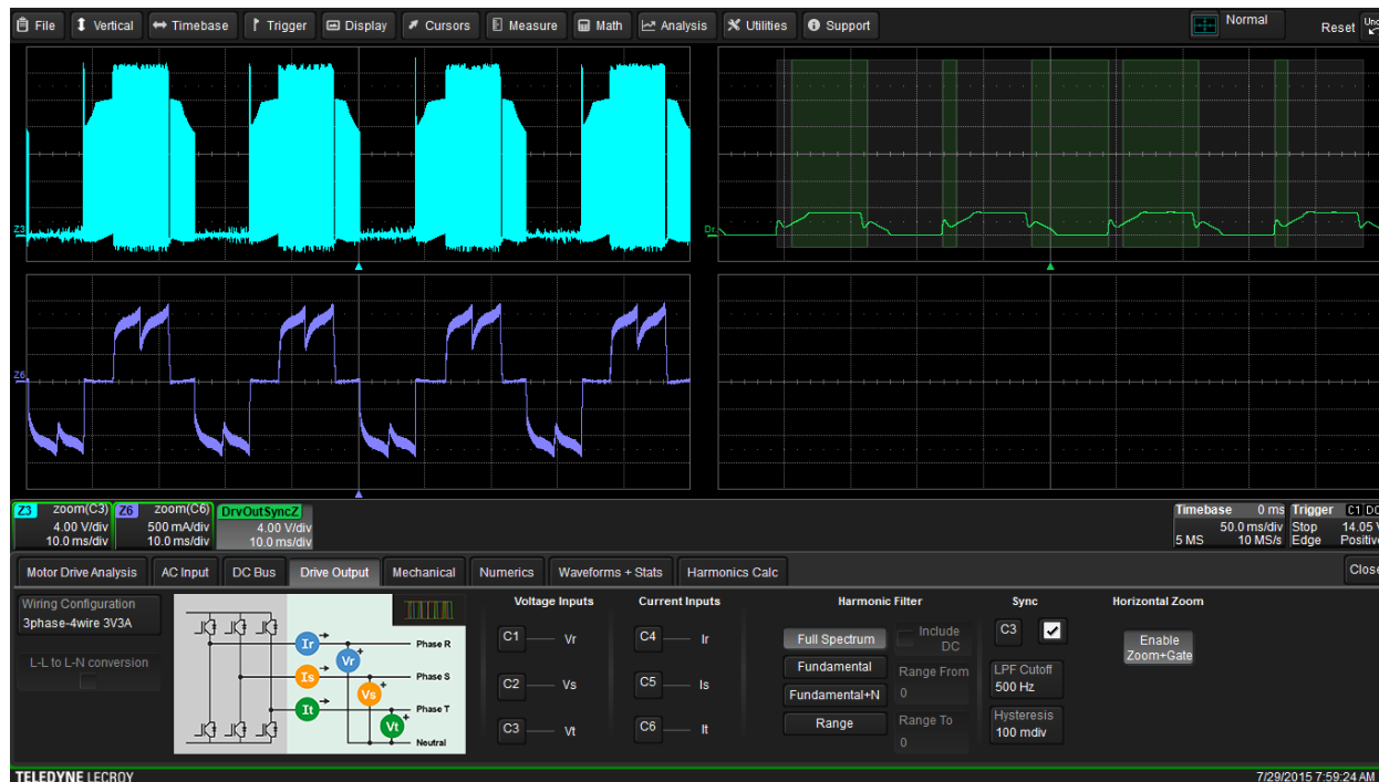
Figure 157: A line-to-reference voltage (Z3, light blue, upper left) of a low-voltage, BLDC, six-step commutated drive output is chosen as the Sync signal, but the MDA software cannot accurately determine the cyclic period.
