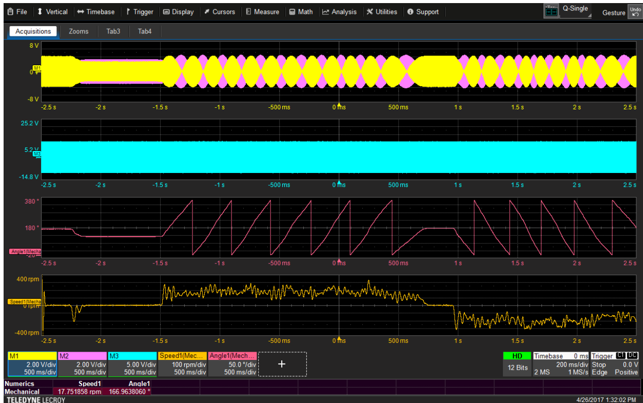
Figure 183: Capture of resolver signals measuring the dynamic movement of a servo motor shaft. Resolver sine (M1, yellow), cosine (M2, magenta), and excitation frequency (M3, or light blue) are shown along with speed and angle mean values and waveforms.
