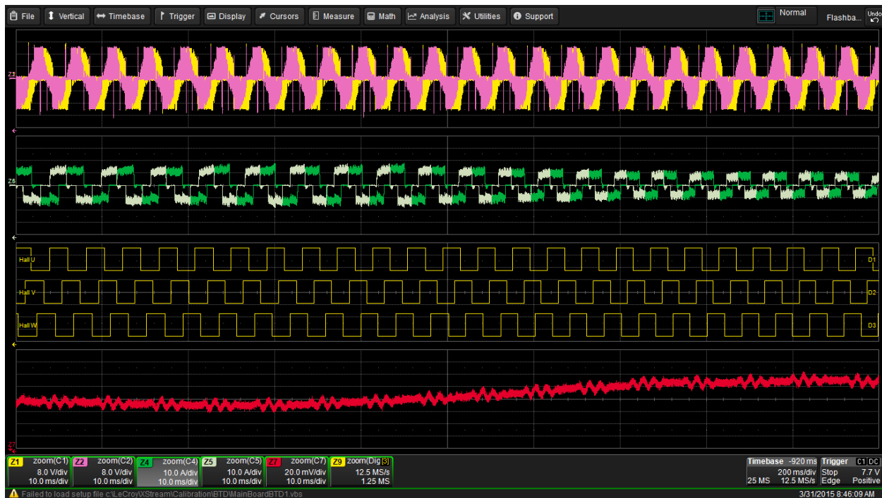
Figure 139: Two of three line-to-line drive output voltages (Z1, yellow and Z2, magenta) with drive output motor line-currents (Z4, gray and Z5, green); digital Hall-sensor signals (Hall U, V, and W, yellow traces); and torque sensor signals (Z7, red) are shown for a six-step commutated closed-loop (sensored) control system.
