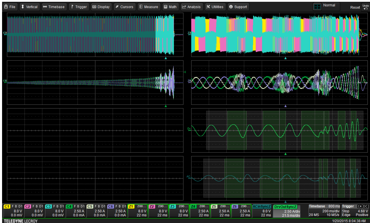
Figure 162: Changing zoom position changes display of all zoomed waveforms, including Sync signals.
