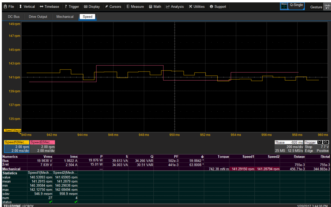
Figure 200: Angle tracking observer applied to Hall Sensor digital signals.
