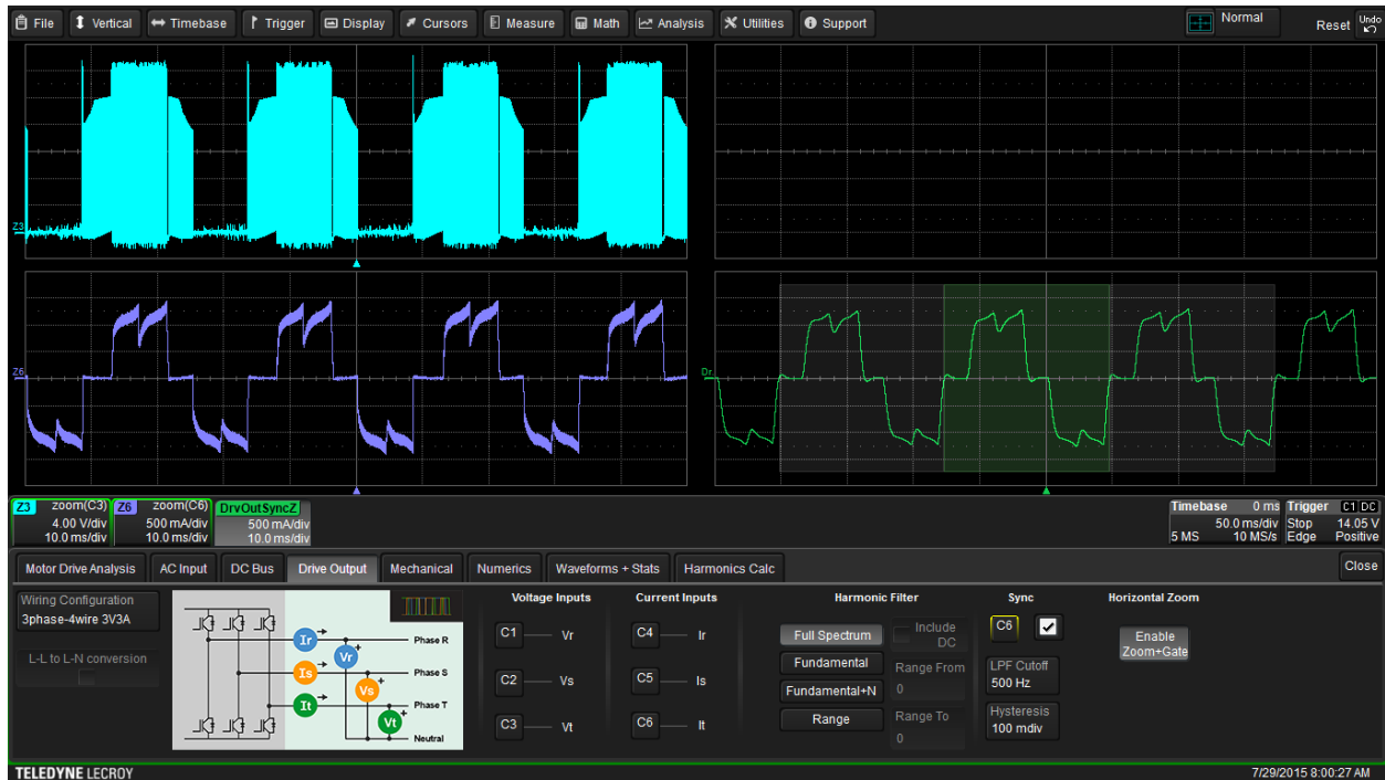
Figure 158: When the line-current waveform is selected as the Sync signal, the MDA is able to correctly determine the cyclic period using default settings.
