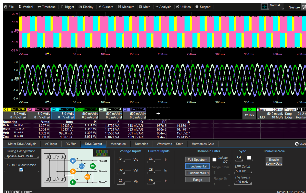
Figure 169: Numerics data calculated for only the fundamental. Note that only the table changes.
