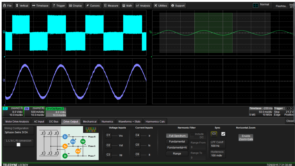
Figure 152: A single line-to-line voltage (Z3, light blue, upper left) and line-current output (Z6, purple, lower left) of a low-voltage vector FOC drive. The filtered Sync signal with cyclic period overlays appears as DrvOutSyncZ (green, upper right.)
