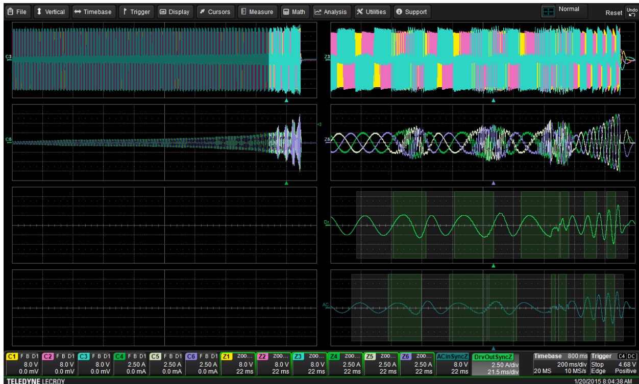
Figure 163: Adjusting filters reveals DriveOutSyncZ (C4, second waveform from the bottom on the lower right) is the better choice Sync signal.
