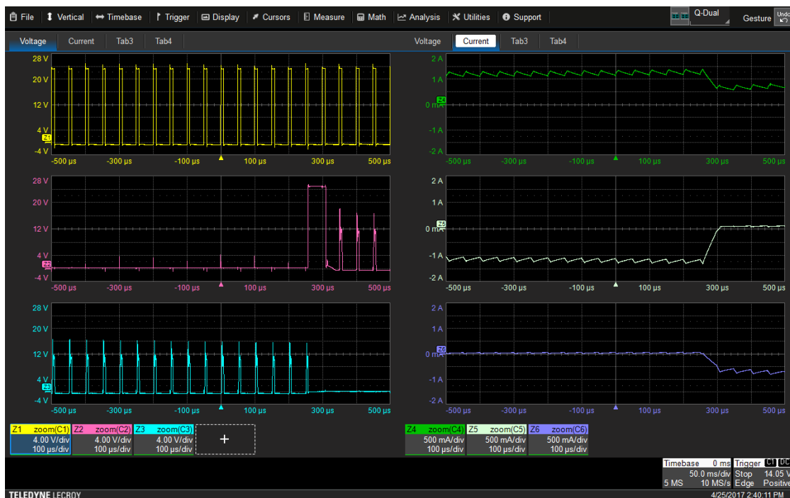
Figure 136: By zooming in on the trapezoidal waveforms, the underlying PWM signals become visible.
