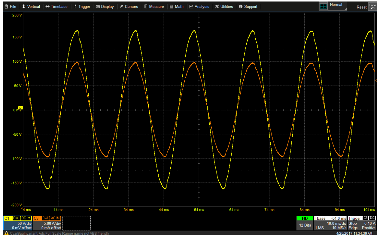
Figure 28: AC line current (orange trace) and 120 Vac voltage (yellow trace) waveforms captured with a Teledyne LeCroy 8-channel, 12-bit Motor Drive Analyzer. The two signals are in phase as expected with a resistive load.
