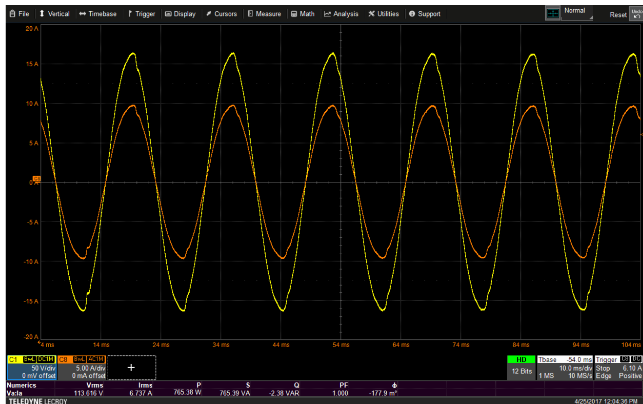
Figure 49: Line-to-neutral voltage waveform and the associated current waveform for a linear load are shown with the Numerics calculation table, which displays various power-related parameters for these waveforms.
