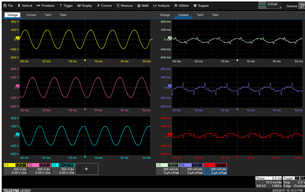
Figure 62: Measurement of voltage and current signals for a three-phase, four-wire AC input to a motor drive.
