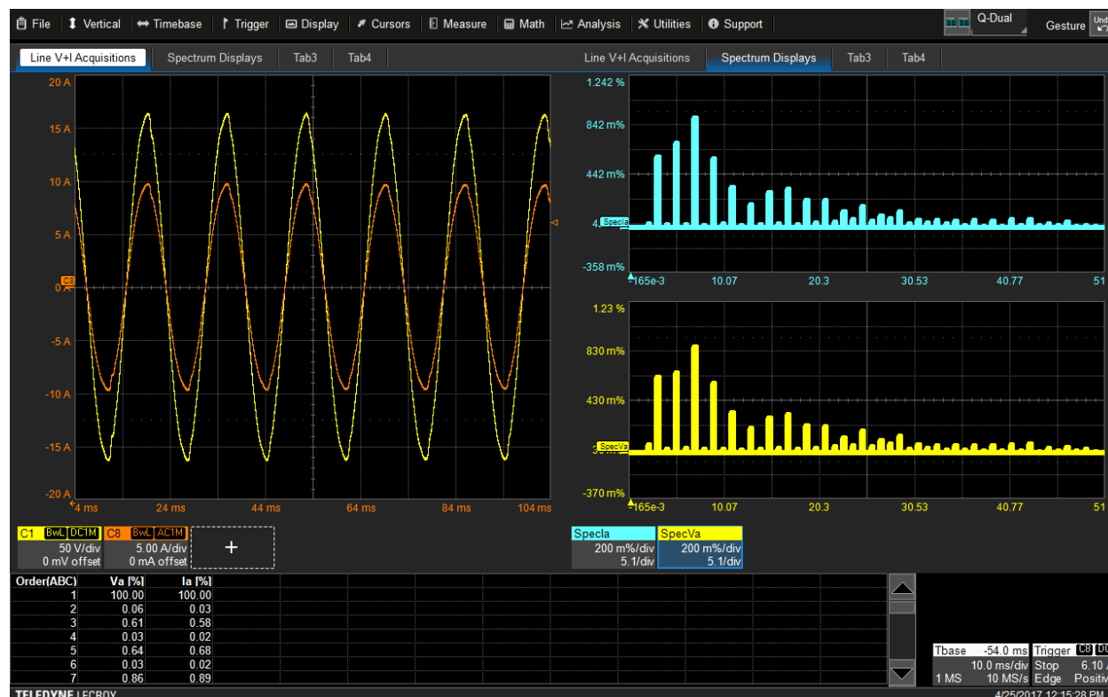
Figure 53: Harmonic order calculations (as percentages of the fundamental) and spectral displays for the voltage and current waveforms.
