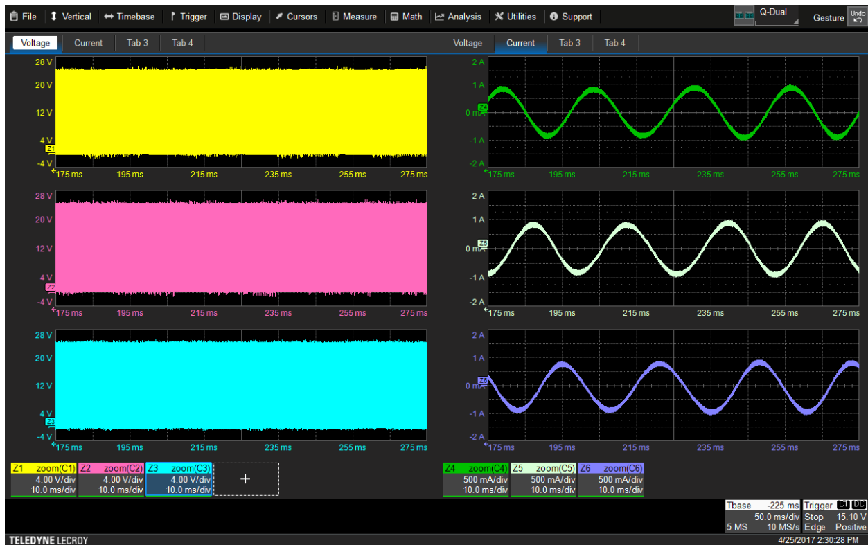
Figure 142: Motor drive line-to-reference output voltages and currents from a small, sensorless vector FOC drive output.
