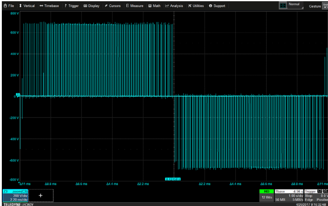
Figure 98: An output waveform produced by an H-bridge. Because of the +V_{dc} and -V_{dc} levels, the H-bridge is also referred to as a two-level inverter or two-level drive.
