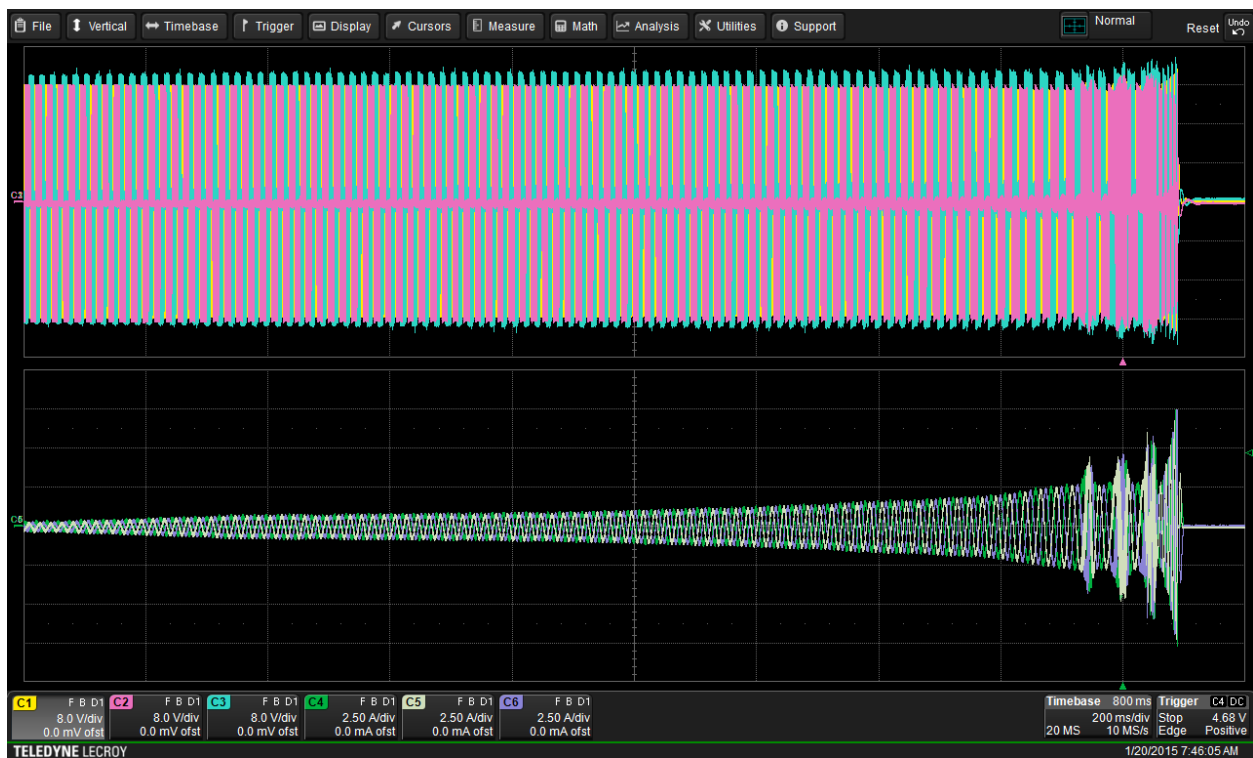
Figure 160: Initial display of input source waveforms for sine-modulated, three-phase drive.
