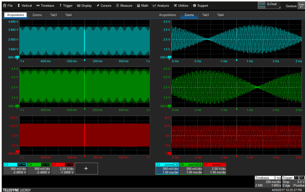
Figure 179: Measurement of resolver signals using the Motor Drive Analyzer. On the left side of the display, we see full 2-s acquisitions of the excitation reference (C7, bottom left), the sine output (C3, top left) and cosine output (C4, middle left). Zooms of the full acquisitions appear on the right.
