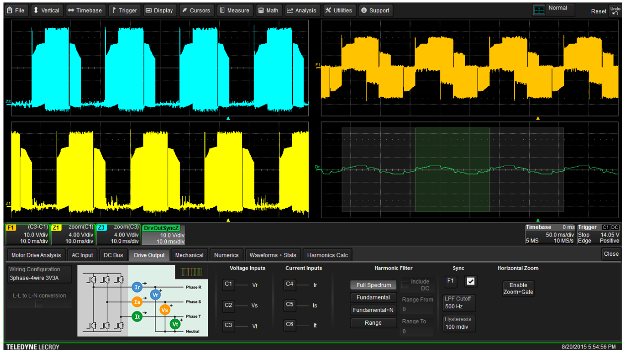
Figure 159: A Math function within the MDA takes the difference between the two line-to-reference waveforms shown on the left and uses this difference waveform as the Sync signal shown on the lower right.
