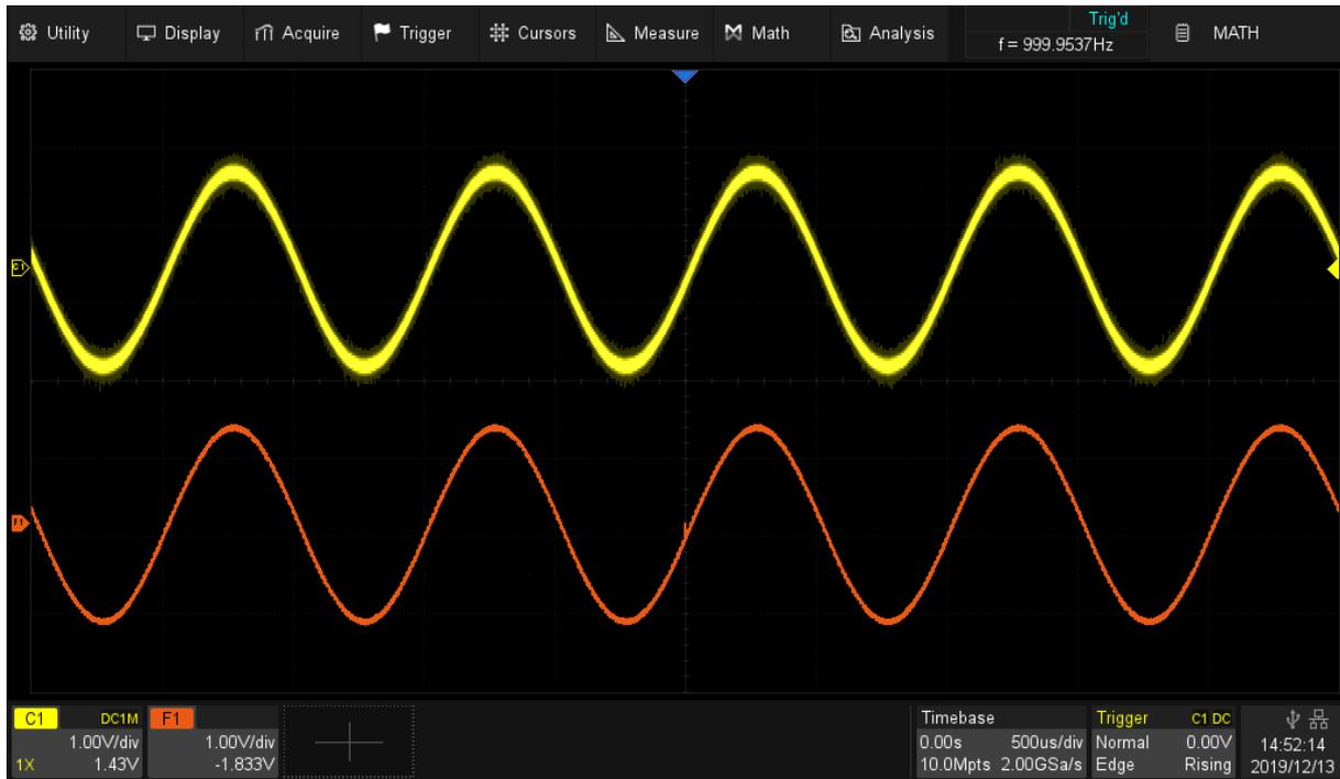
Note: Average acquisition is only valid for repetitive periodic signals, and it is important to ensure that the waveform is triggering in a stable way when using average mode.
