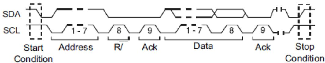
**EEPROM** — The trigger searches for the EEPROM control byte value 1010xxx on the SDA bus. And there is a Read bit and an ACK bit for the EEPROM. Set the data value and compare type according to Data1 and Limit Range. If EEPROM’s data is greater than (less than, equal to) Data1, the oscilloscope will be triggered at the edge of ACK bit after the Data byte. It’s not necessary for a Data byte to follow the EEPROM.
