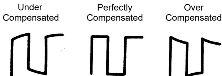
5. Use a non-metallic screwdriver to adjust the low-frequency compensation adjustment hole on the probe until the waveform displayed is as the “Perfectly compensated” in the figure above.
