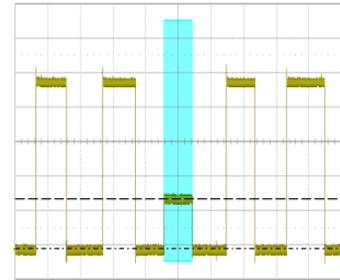
The input signal is a 2 V periodic square wave, in which every 10ms there is a runt pulse with a height of 1/3 of the normal amplitude:
