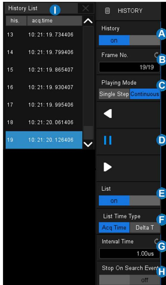
The oscilloscope automatically stores acquired frames. It can store up to 90,000 frames but the number varies due to the channel memory depth and timebase settings. Turn on history mode, then the stored frames can be recalled and measured.
