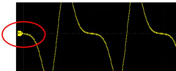
Channel Offset Indicator with a channel number shows the offset position of the corresponding channel.
