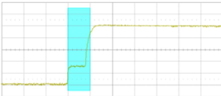
With a simple edge trigger, it is unlikely to trigger consistently on this anomaly.
