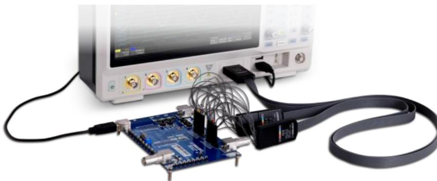
To connect the logic probe: Insert the probe, with the correct side facing up, until you hear a “click”.
