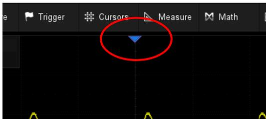
Trigger Delay Indicator locates where the waveform triggers on the horizontal axis.
