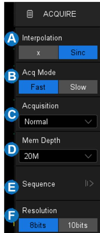
Memory Depth: The maximum memory depth that can be supported. According to the formula "acquisition time = sample points x sample interval", setting a larger memory depth can achieve a higher sample rate for a given time base, but more samples require more processing time, degrading the waveform update rate. With 200 Mpts memory depth, the T3DSO2000A can still run at full sample rate (2 GSa/s) even when set to the 10 ms/div timebase.
