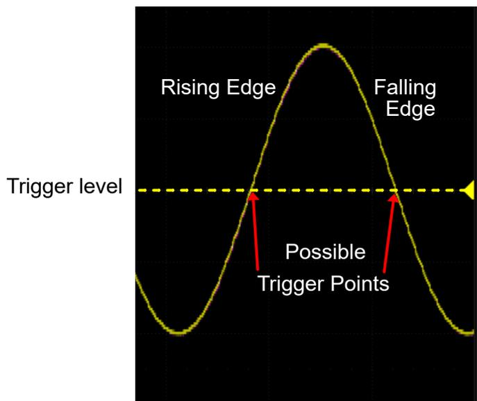
Touch the Source area to select trigger source, and touch the Slope area to select rising, falling or alter.
