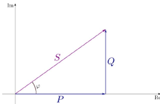
$$P: \text{Active Power} = \frac{1}{N} \times \sum_{i=0}^{n-1} V_i \times I_i$$
