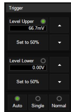
The lower level should always be less than or equal to the upper level. In the trigger descriptor box, the lower level is displayed.
