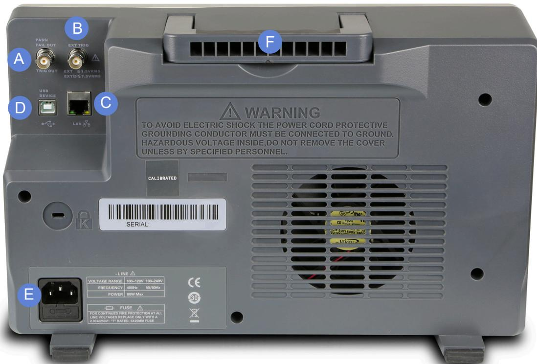
A. Auxiliary Out: Outputs the trigger indicator. When Pass / Fail is enabled, outputs the pass / fail signal.
