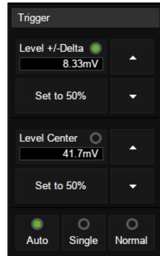
**Note:** "Level +/-Delta" represents half of the actual window area. For example, when the value is 200 mV, it actually represents a range of  $\pm 200$  mV, which is a 400 mV window.
