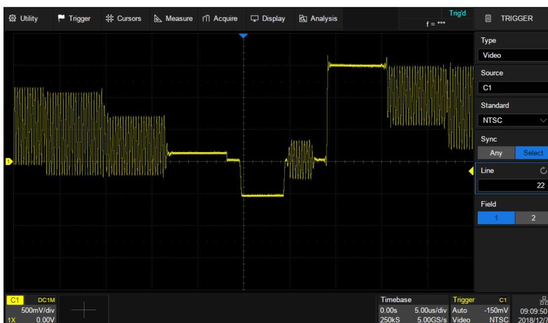
Trigger on a Specific Line of Video(NTSC)
