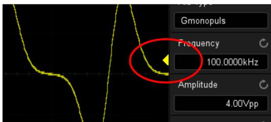
Trigger Level Indicator shows the level where the waveform triggers on the vertical axis.
