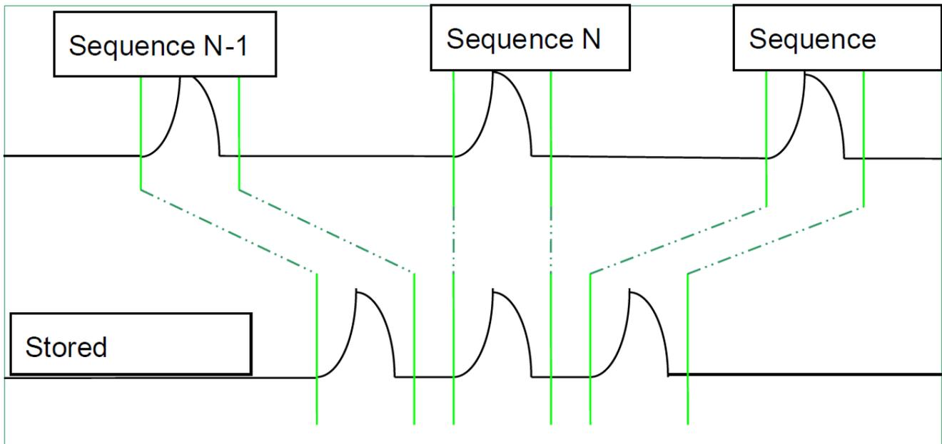
The T3DSO2000A can achieve a minimum  $2\mu\text{s}$  trigger interval in Sequence mode, corresponding to a waveform update rate of 500,000 wfm/s.
