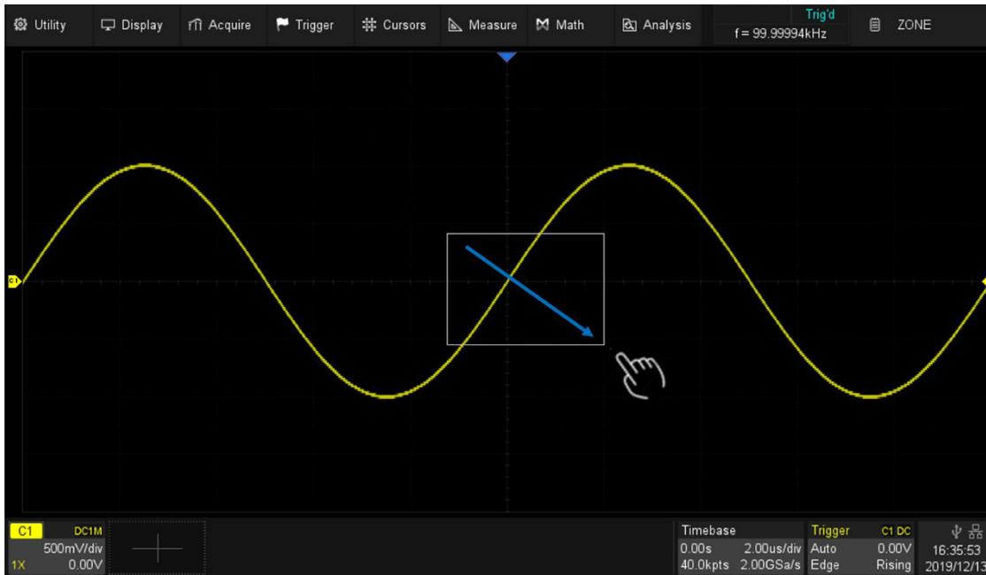
When the users finger moves off the screen, a menu pops up for selecting the zone and setting the zone properties.
