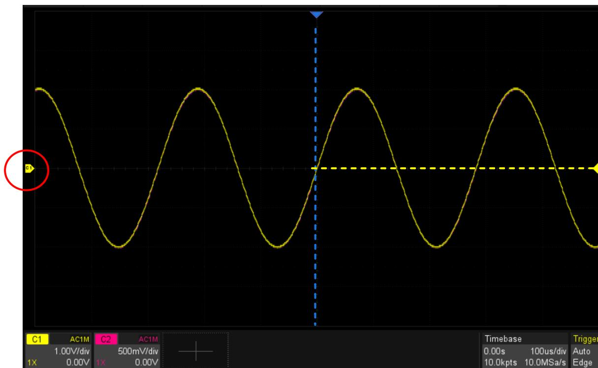
In some special trigger, the system will automatically set the trigger level, such as using AC Line as the trigger source.
