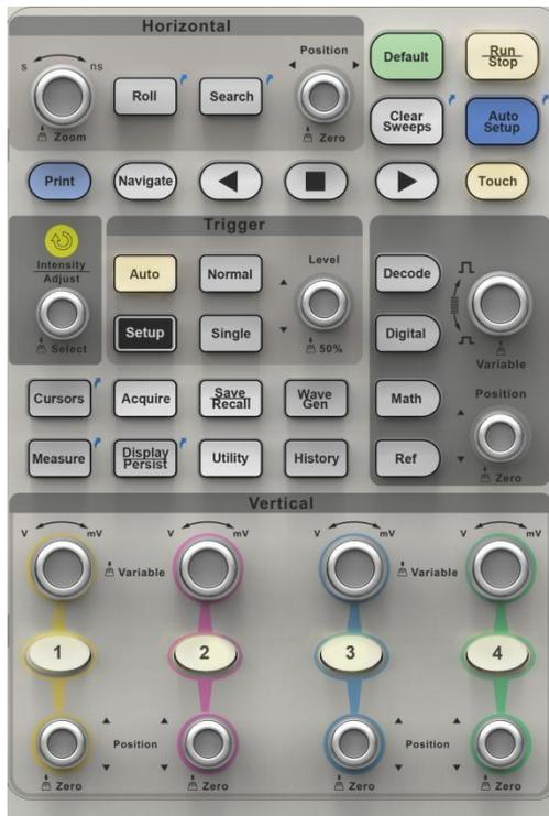
The front panel is designed to operate the basic functions without having to open the software menu. Most of the front panel controls duplicate functionality available through the touch screen display, but it is quicker to use the front panel controls.
