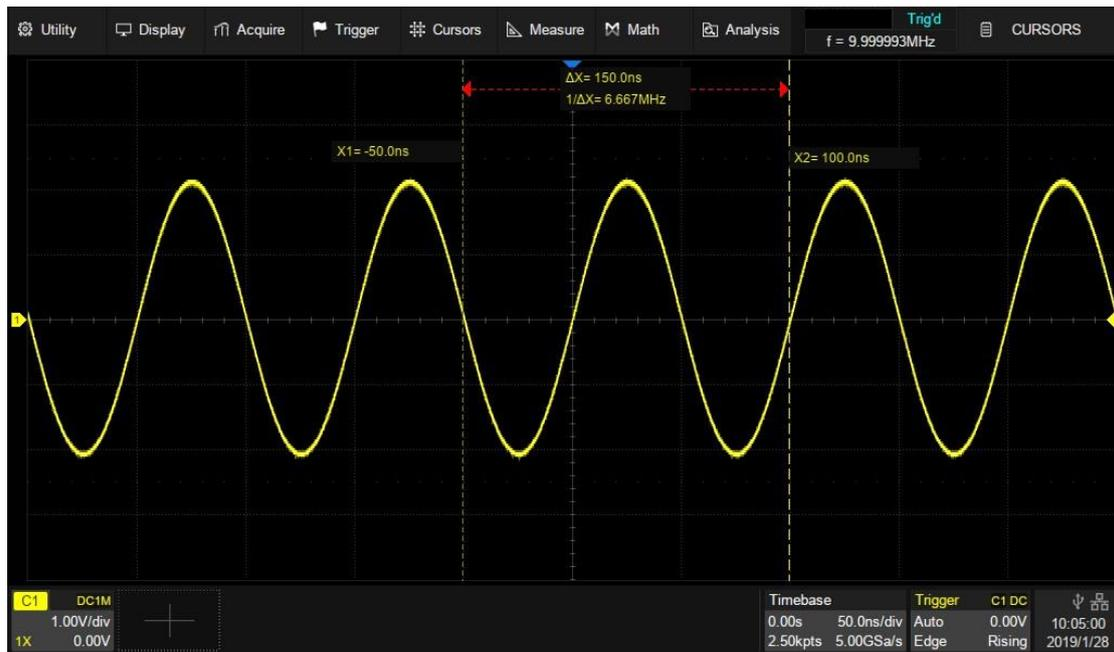
Timebase =  $50\text{ns/div}$  ,  $X1 = -50\text{ns} = -1\text{div}$  ,  $X2 = 100\text{ns} = +2\text{div}$
