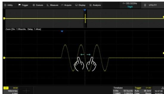
Adjust the horizontal scale of Zoom window by horizontal pinch and spread in the zoom area of the main window or in the Zoom window
