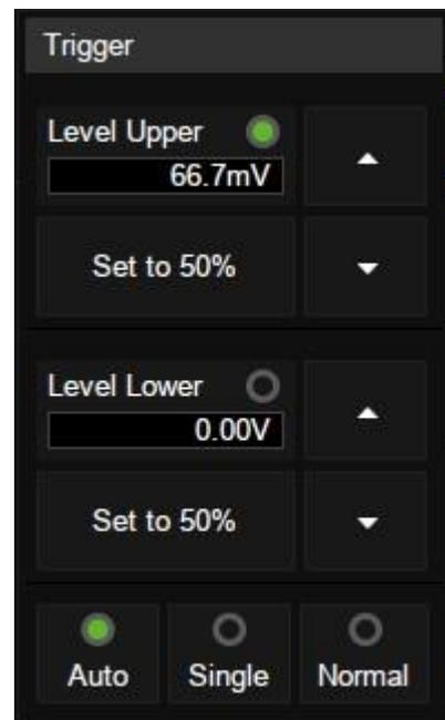
1. Touch the **Level Upper** area in the quick menu to select the upper level, and then set the level value by the virtual keypad or the Level knob on the front panel. To set the lower level is the similar.
