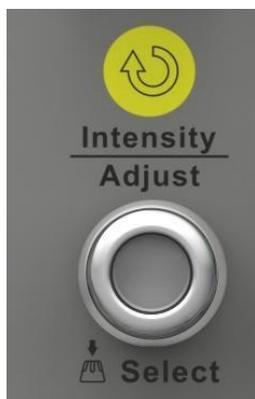
When the parameter setting area is highlighted, you can use the Universal Knob to set the parameter. Press the knob to select an option from the list. The default function of the Universal Knob is to adjust intensity of the waveform traces.
