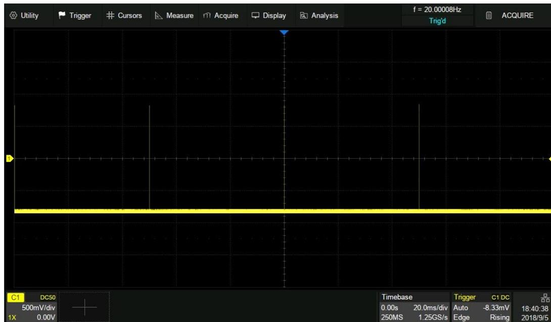
In normal mode, 5 pulses can be obtained on the screen with the sample rate of 1.25 GSa/s at the maximum memory depth.
