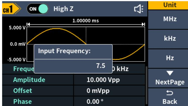
Figure 4-4: Use numeric keypad to set the frequency
