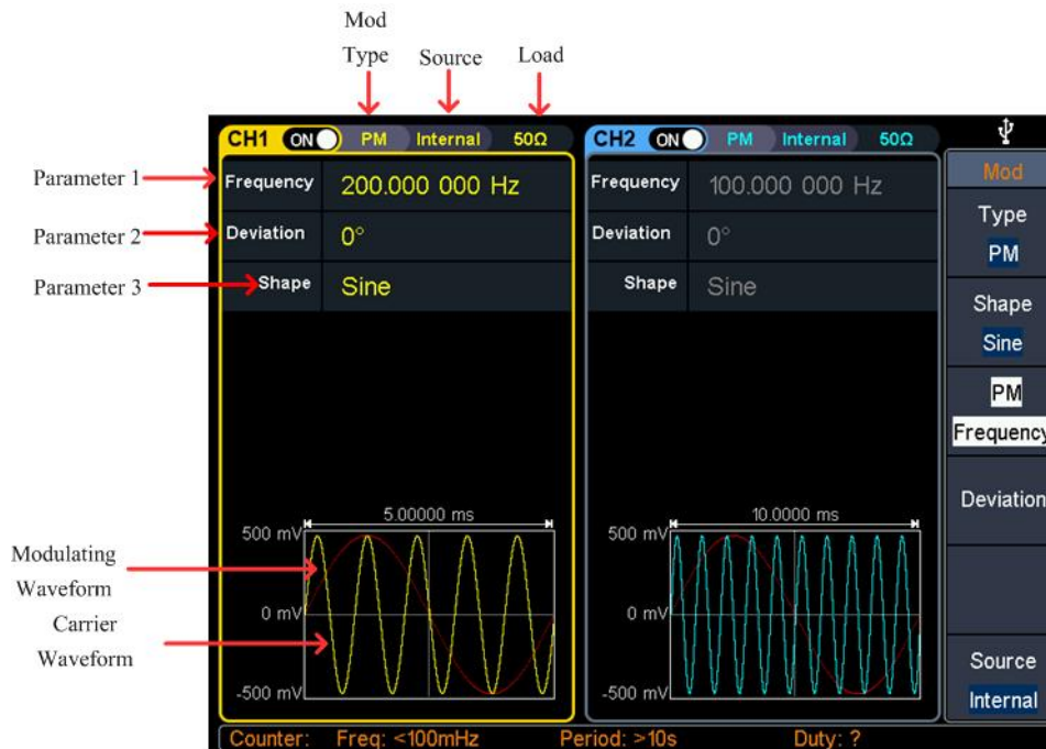
Figure 4- 13: Phase modulation user interface
