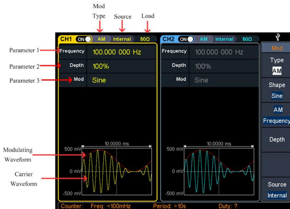
Figure 4- 11: Amplitude modulation user interface
