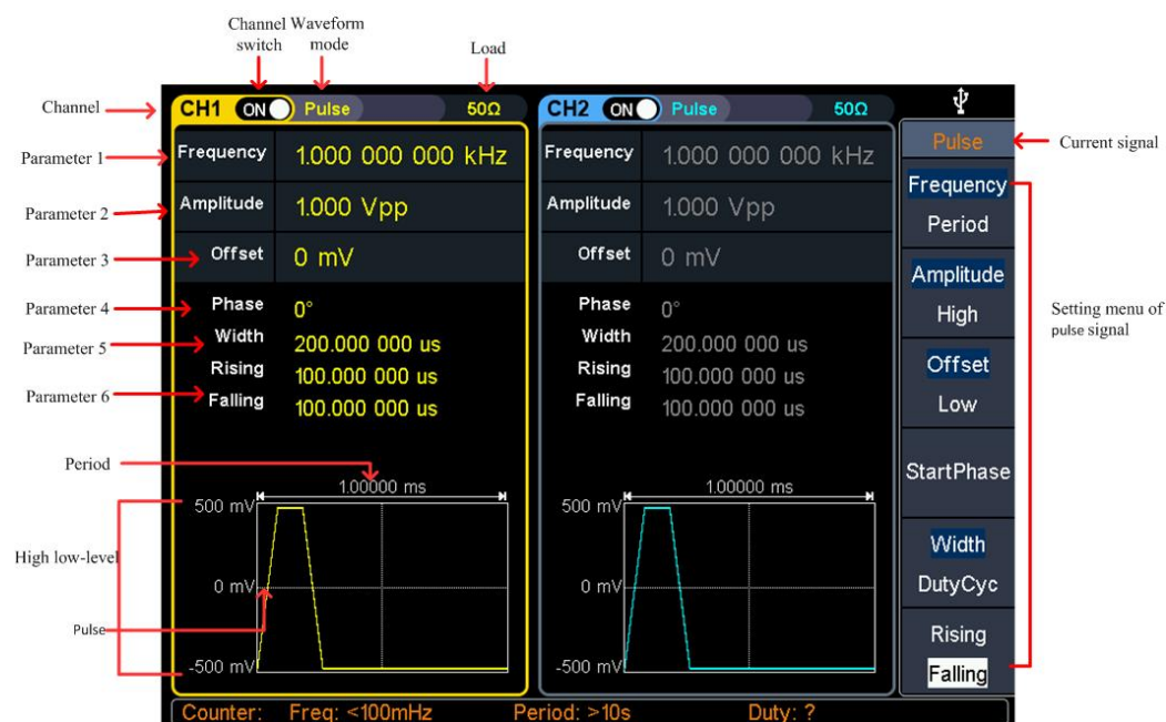
Figure 4- 6: Pulse wave user interface
