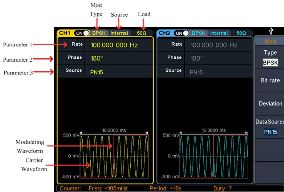
Figure 4- 20 Binary phase shift keying user interface
