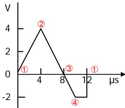
**Note:** As can be seen from the above figure, the waveform editor will always connect from the first point to the voltage level of the last point to create a continuous waveform.
