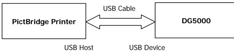
Set the Device Type to “Printer” (refer to **To Set USB Device Type**) and press **Pict Bridge** to enter the setting interface.
