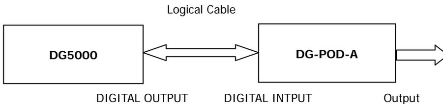
When the connection succeeds, if the system detects a digital module, the shortcut will be automatically switched to “Digital”. To edit digital waveform data, press **Utility** → **Digital** → “Power On” → **User\***.
