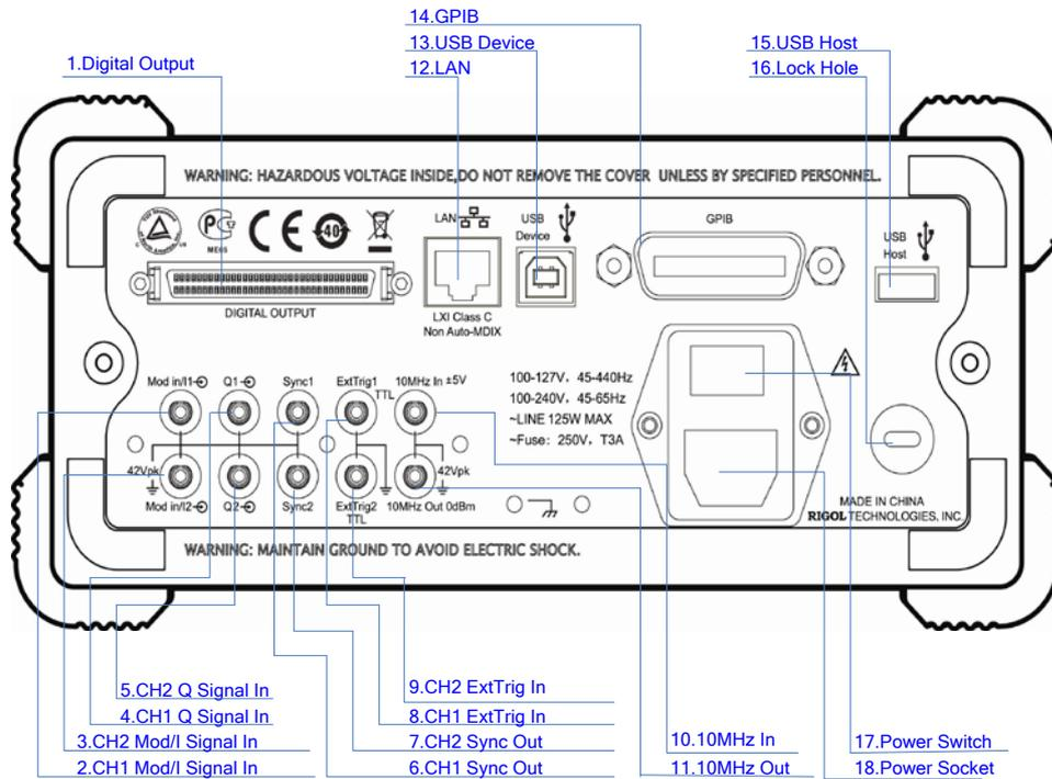
Figure 1-3 Dual-Channel Model Rear Panel Overview
