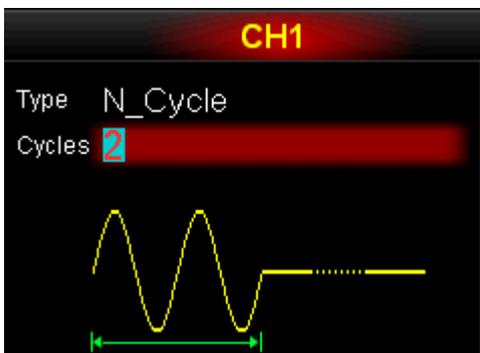
N Cycle Burst could be triggered by "Internal", "External" or "Manual" source. You can
