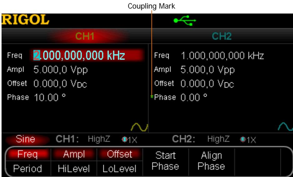
Figure 10-2 Channel Coupling
