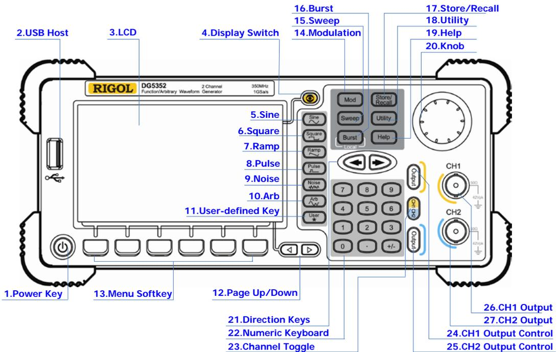
Figure 1-1 Dual-Channel Model Front Panel Overview
