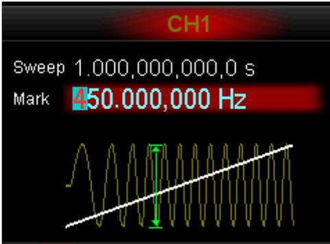
The generator will renewedly sweep and output with the specified “Start Frequency” once the Mark Frequency is changed.
