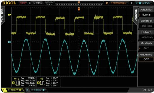
Built-in dual-channel 25 MHz source (MSO/DS2000A-S)
