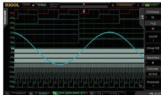
Deeper memory depth for the digital channels, serial bus triggering and decoding for digital channels
