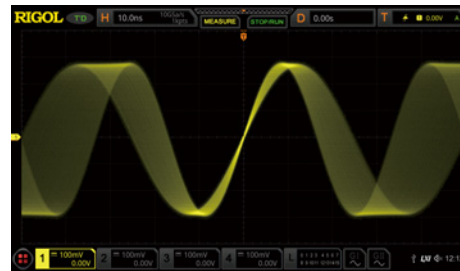
Changes of each frame of waveforms of the sweep signal can be clearly observed in high refresh mode.
