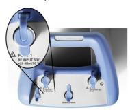
Connect a cable or DUT to the RF input with an N connector. Use a cable to connect the DUT to the R&S FSH, if necessary.
