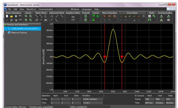
EasyWaveX is an arbitrary waveform software platform that supports waveform creation and editing. It features manual drawing, as-well-as line, equation, and coordinate editing modes. It is also a convenient way for users to edit their own arbitrary waveforms.
