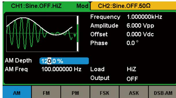
SDG2000X supports plenty of modulation types, such as AM, FM, PM, FSK, ASK, PSK, DSB-AM, and so on. The modulation source can be configured as "Internal" or "External".
