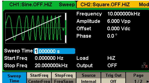
SDG2000X supports two Sweep modes, "Linear" and "Log". Two Sweep directions, "Up" and "Down" and three Sweep sources, "Internal", "External" and "Manual".
