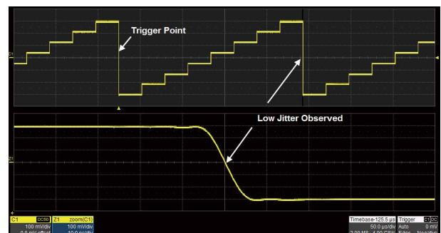
As with EasyPulse, TrueArb effectively overcomes the defect that DDS may cause the one-clock-jitter in arbitrary waveforms.
