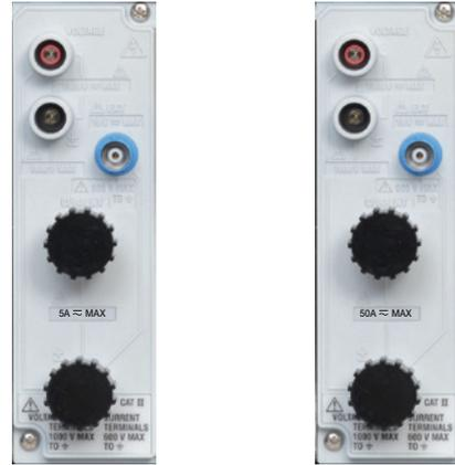
Both 5 A and 50 A input elements can be installed in a single unit. This enables engineers to use a single WT1800E for multiple applications such as standby power measurement and the evaluation of various operating modes of the device under test.
