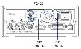
TRIG IN may be used as external trigger input in the following cases. The polarity setting can be changed.
