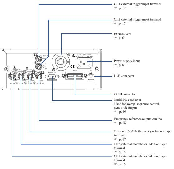
Figure 3-4. Rear Panel of FG420
