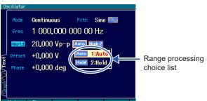
Select the range icon on the right of the amplitude display to display the current range under that icon. The current range is displayed as a combination of maximum output voltage Vp-p and the amplitude attenuator.
