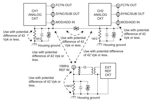
Figure 3-7. Cautions on Floating Ground Connection for FG420
