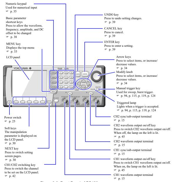
Figure 3-3. Front Panel of FG420
