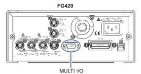
MULTI I/O can be used for sweep control and sequence control. It outputs the step synchronization code for the sequence.
