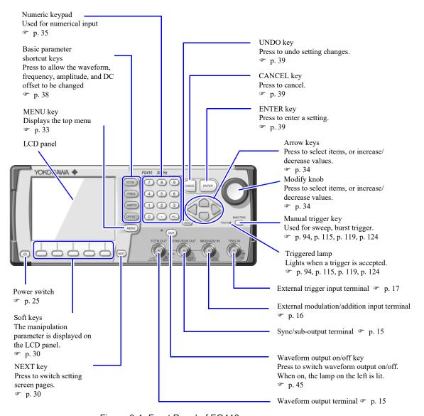
Figure 3-1. Front Panel of FG410
