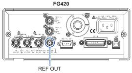
Use REF OUT to unify the frequency and phase for multiple FG410, FG420 units.
