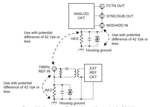
Figure 3-6. Cautions on Floating Ground Connection for FG410
