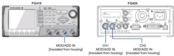
When the modulation source is external, except for FSK and PSK, an external modulation signal is input. In the case of the FSK and PSK, the external trigger input is used as external modulation signal input.
