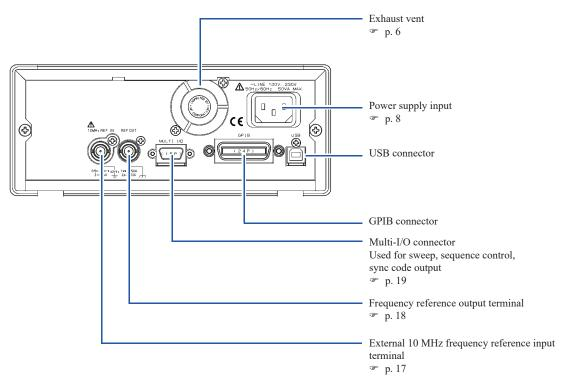
Figure 3-2. Rear Panel of FG410
