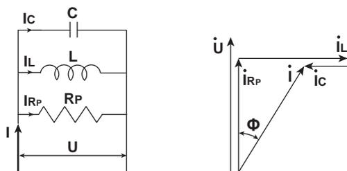
The relationship between resistance  $R_P$ , reactance  $X_P$ , and impedance  $Z$  is expressed by the equations below.
